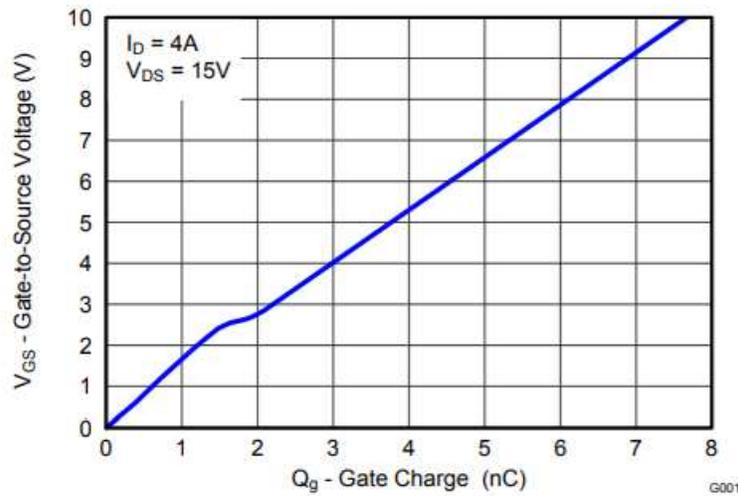
Figure 2. MOSFET Gate Charge
