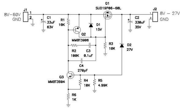
**Figure 2-2. Discrete Voltage Clamping Circuit**
