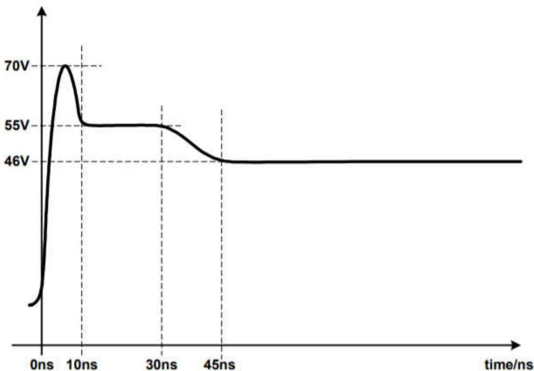
**Figure 2-1. Example of a Fast Line Voltage Transient That Can Damage PLC Circuits**
