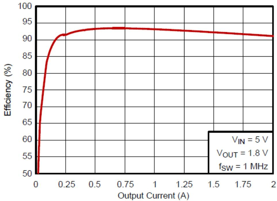
Figure 3-1. Efficiency Curve of TPS54218
