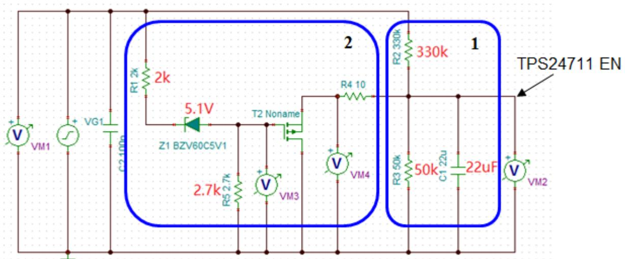
The circuit 1 is a resistor divider and ceramic capacitor to achieve insertion turn ON delay function. When board is plugged in, TPS24711 EN pin voltage is controlled by R2, R3 and C1. EN typical rising threshold voltage is 1.3 V with 50 mV hysteresis.
