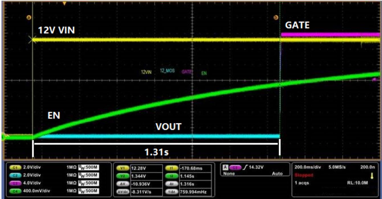
Figure 7. Fast Turn OFF Test Result
