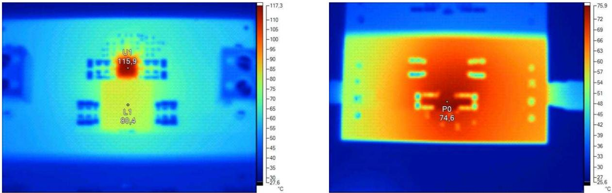
Figure 16. Layout 1 - Single Sided, All Components Top Side
