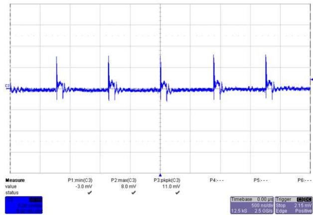
Figure 8. Layout 2 - Output Ripple, 5 mV/div, 12 V to 1.2 V at 8 A
