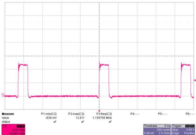
Figure 14. Switch Node Waveform, Layout 2
