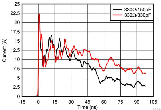
**Figure 2-2. 330-Ω, 5-kV Contact Discharge**
