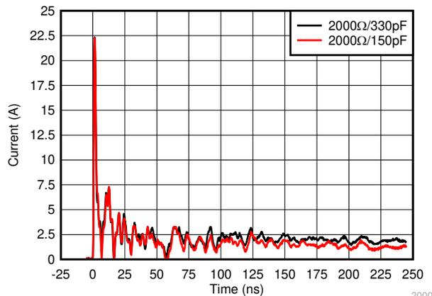
**Figure 2-3. 2000-Ω, 5-kV Contact Discharge**
