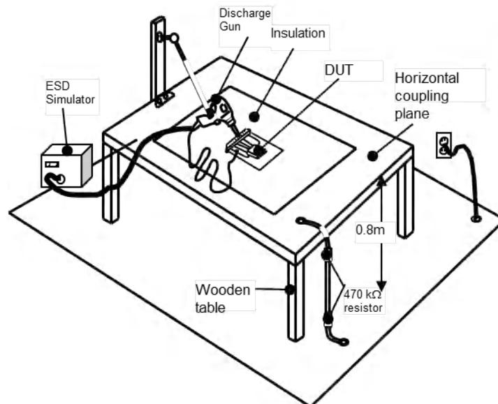
**Figure 3-1. ISO 10605 Basic Table Setup**
