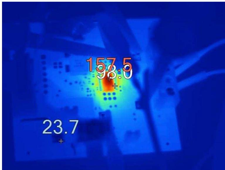
**Figure 4. Board 1 Thermal Image for Top of Case Temperature**
