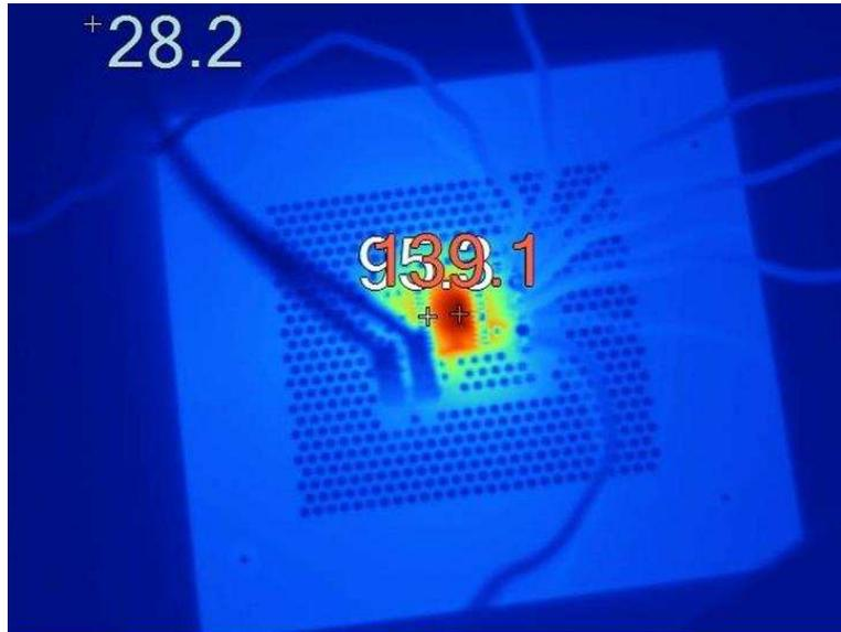
Figure 5. Board 2 Thermal Image for Top of Case Temperature
