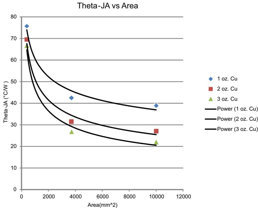
**Figure 6. Thermal Simulation Data Comparing Board Size and Copper Weight**
