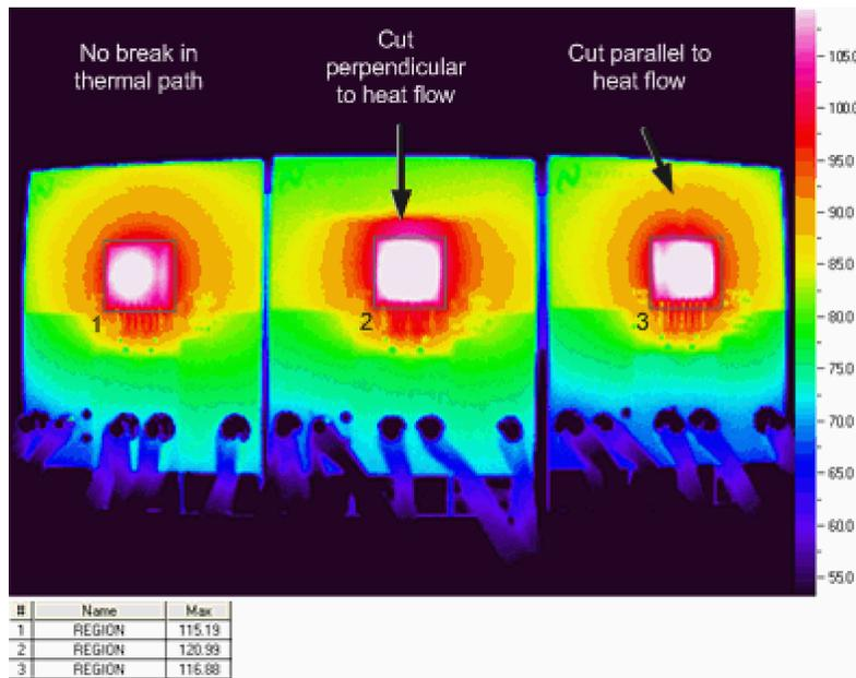
Figure 7. Hot Spot Created When a Break is Created in the Thermal Path
