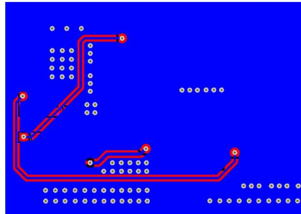
**Figure 7. Bottom PCB Layout**
