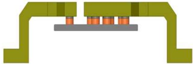
**Figure 4. FCOL SOT23 Package Cross-Sectional View**
