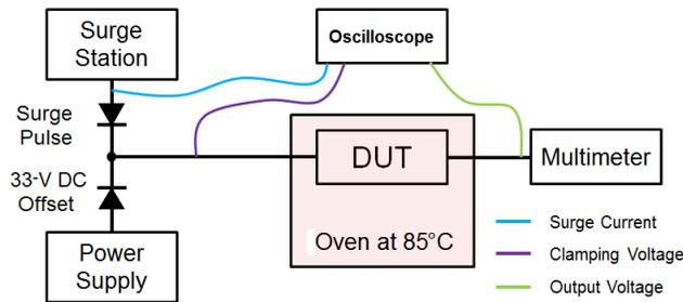
Figure 9. Test Setup Block Diagram
