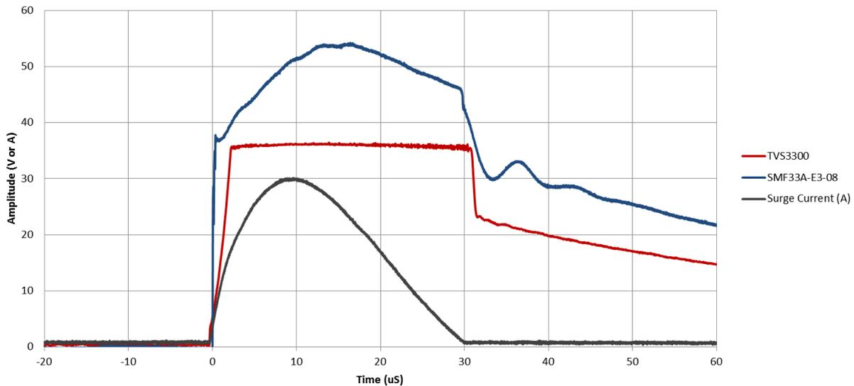
**Figure 5. 8/20  $\mu$ s Surge Clamping Waveform of Flat-Clamp Diode vs. Conventional TVS Diode**
