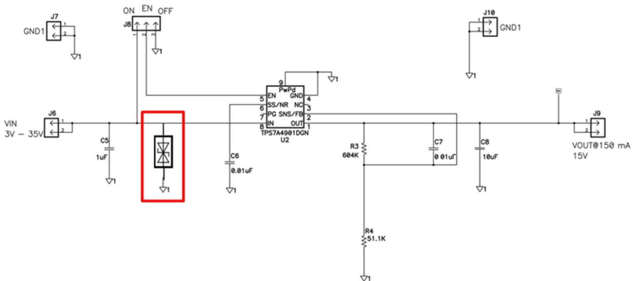
Figure 6. Modified TPS7A4901DGN EVM Schematic
