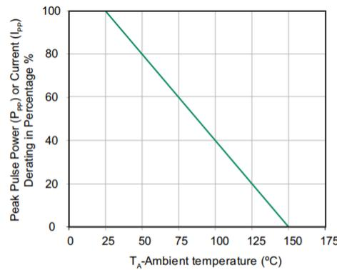
**Figure 3. Littelfuse® SMAJ33A Series Temperature Derating**
