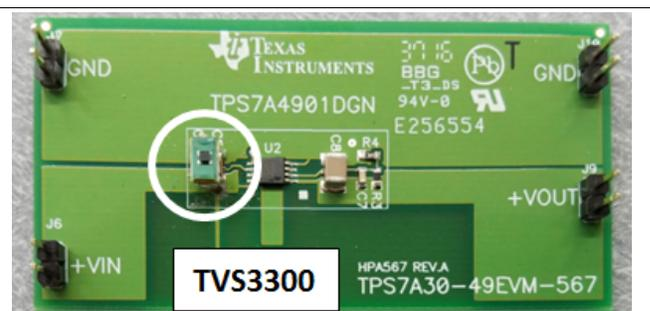
Figure 8. TPS7A4901DGN with TVS3300 on the Input Voltage Line
