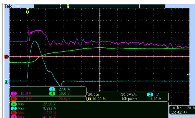
Figure 10. SMAJ33A Protection at 8.38 A at 85°C
