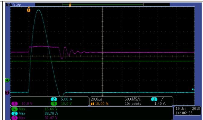
Figure 13. TVS3300 Clamping Waveform at Last Passing Current at 85°C
