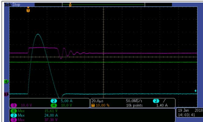
Figure 12. TVS3300 Clamping Waveform at 24 A at 85°C
