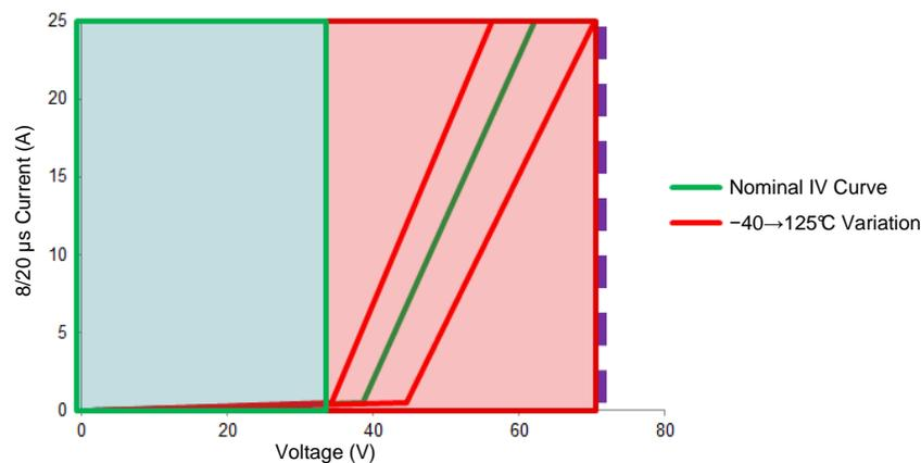
Figure 2. Process and Temperature Variation on SMAJ33A
