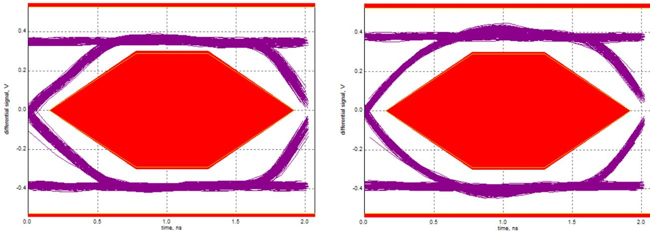
Figure 9. Eye Diagram With and Without LC Network
