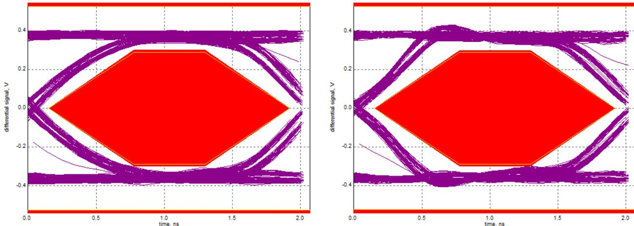
**Figure 14. Eye Diagram With and Without TUSB211**
