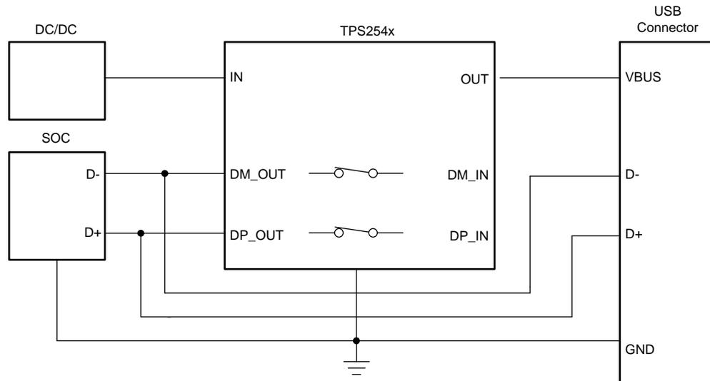
Figure 10. Bypass DP\_IN and DM\_IN
