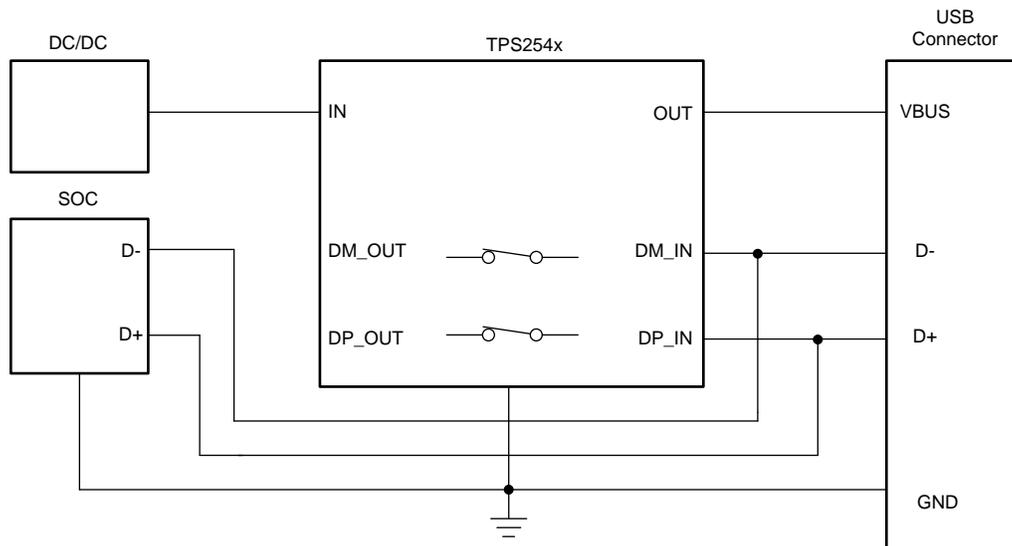
Figure 11. Bypass DP\_OUT and DM\_OUT
