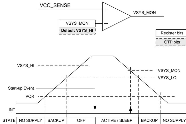
Figure 7. System Voltage Monitor and System State Diagram
