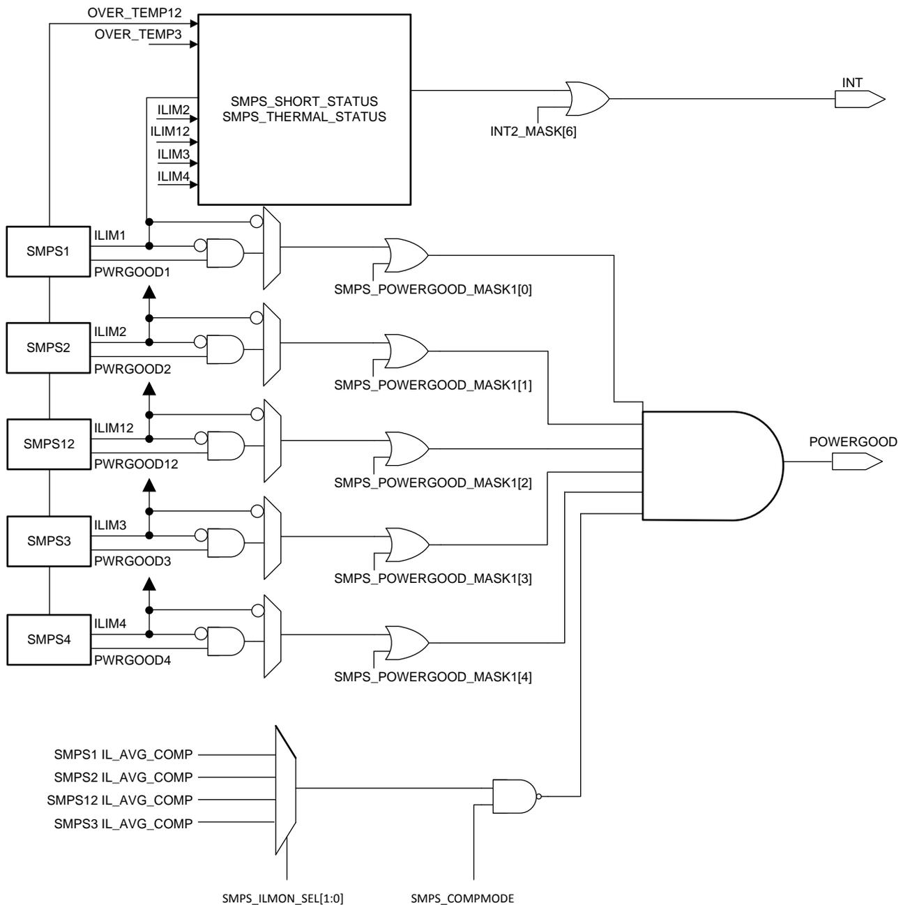
**Figure 9. POWERGOOD Block Diagram**
