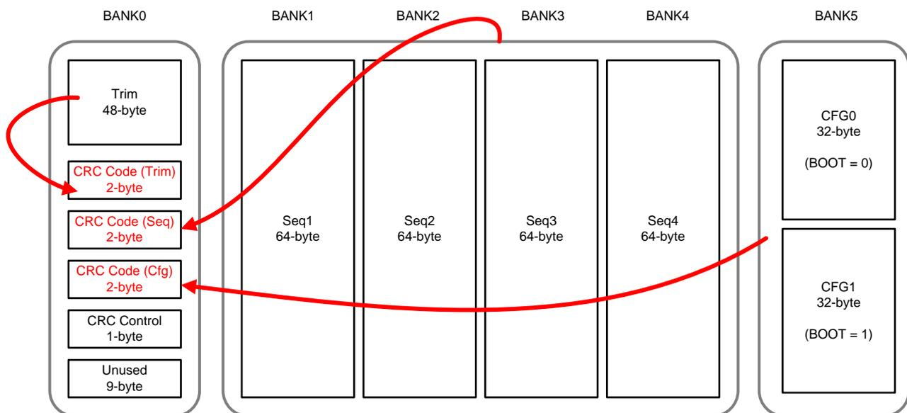
**Figure 6. OTP Register Map Diagram**
