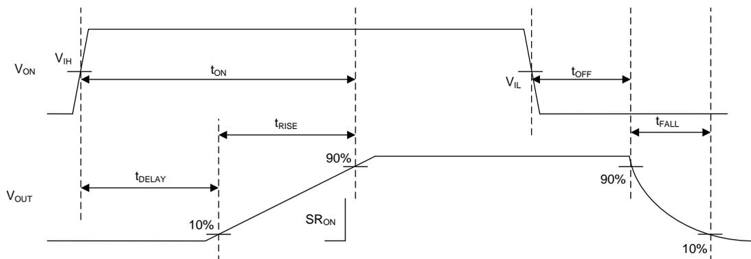
Figure 1.  $t_{\text{DELAY}}$ ,  $t_{\text{ON}}$ ,  $t_{\text{OFF}}$ ,  $t_{\text{RISE}}$ , and  $t_{\text{FALL}}$  Waveforms
