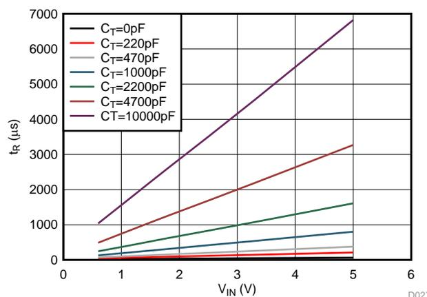
**Figure 11. TPS22958  $t_{\text{R}}$  vs  $V_{\text{IN}}$  With Changing CT**
