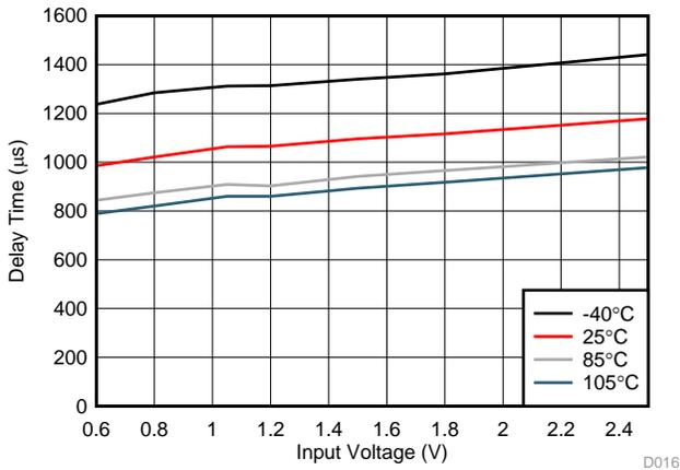
Figure 12. TPS22976  $t_{DELAY}$  vs  $V_{INPUT}$
