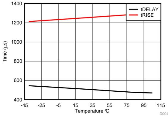
Figure 6. TPS22918  $t_{RISE}$  and  $t_{DELAY}$  Across Temperature
