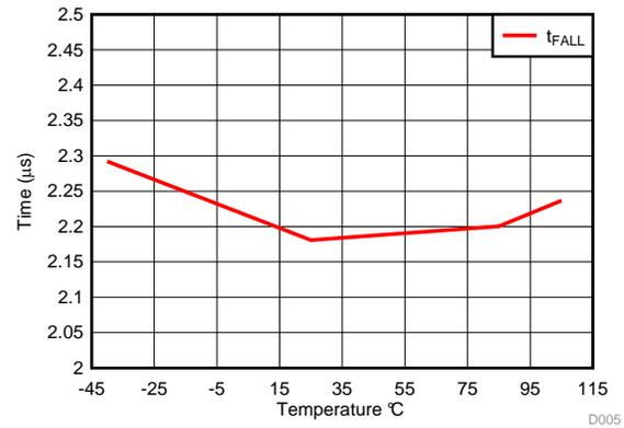
Figure 7. TPS22918  $t_{FALL}$  Across Temperature
