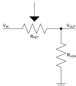
Figure 8.  $R_{FET}$  and  $R_{LOAD}$  Voltage Divider
