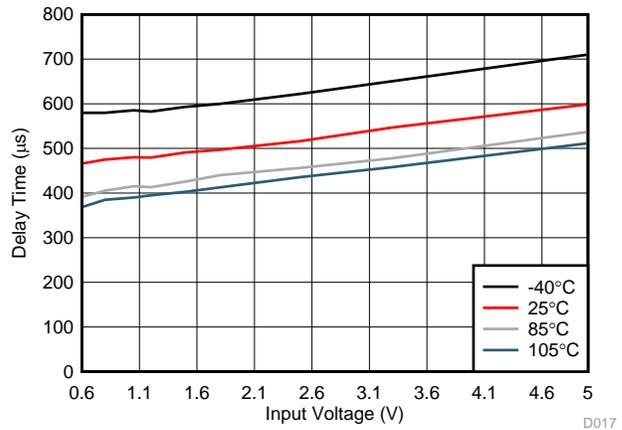
Figure 13. TPS22976  $t_{DELAY}$  vs  $V_{INPUT}$
