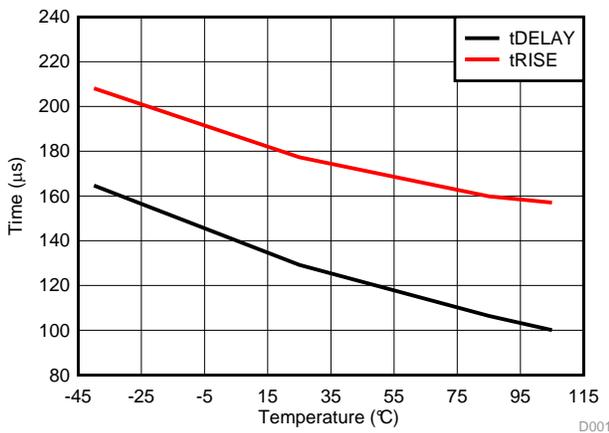
Figure 4. TPS22975  $t_{RISE}$  and  $t_{DELAY}$  Across Temperature
