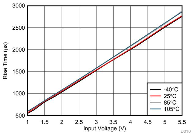
Figure 9. TPS22976  $t_{RISE}$  vs  $V_{INPUT}$
