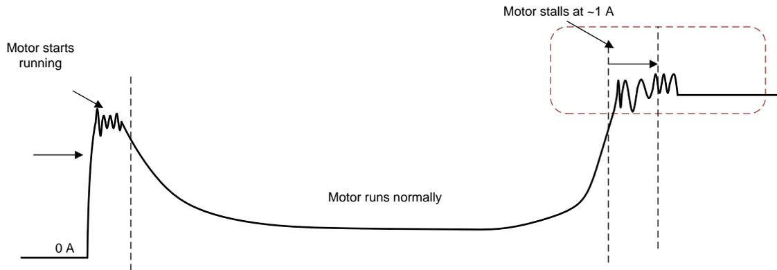
Figure 6. Motor-Current Profile
