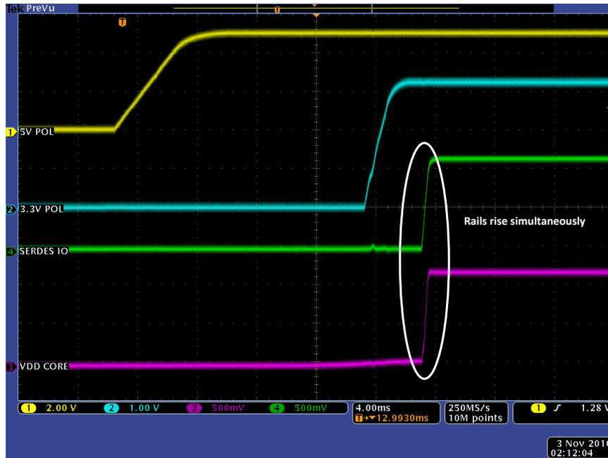
**Figure 3-7. RTG4 Modified Development Board Fulfilling the Second Power-Up Requirement**
