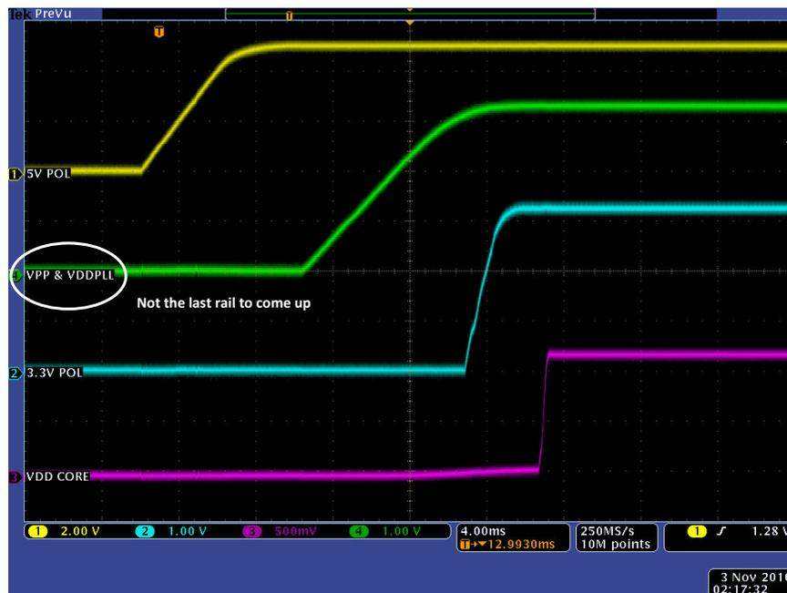
**Figure 3-6. RTG4 Modified Development Board Fulfilling the First Power-Up Requirement**
