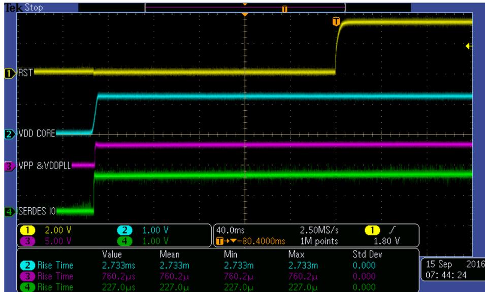
Figure 2-2. RTG4 Development Board Start-up Sequence
