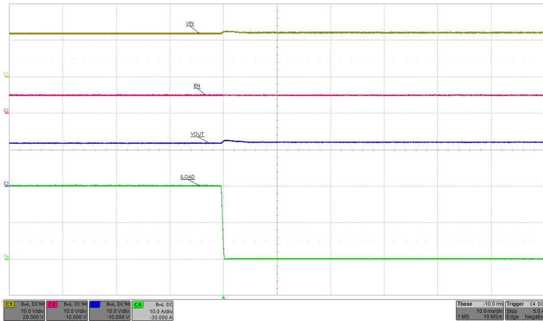
Figure 12. 20-A Load Step-Down Response of Four-Phase eFuse Parallel Configuration
