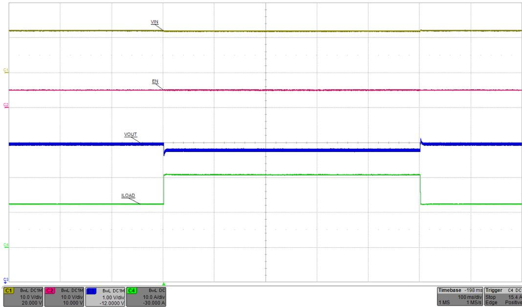
Figure 13. Transient Overload Response of 20-A eFuse
