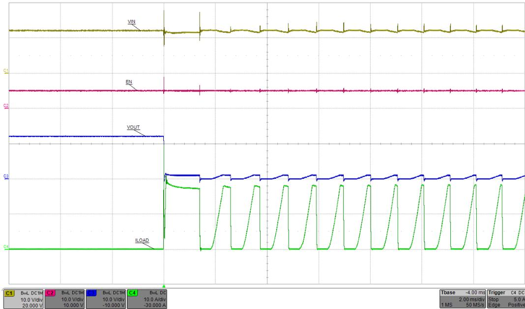
Figure 14. Output Short-Circuit Response of 20-A eFuse
