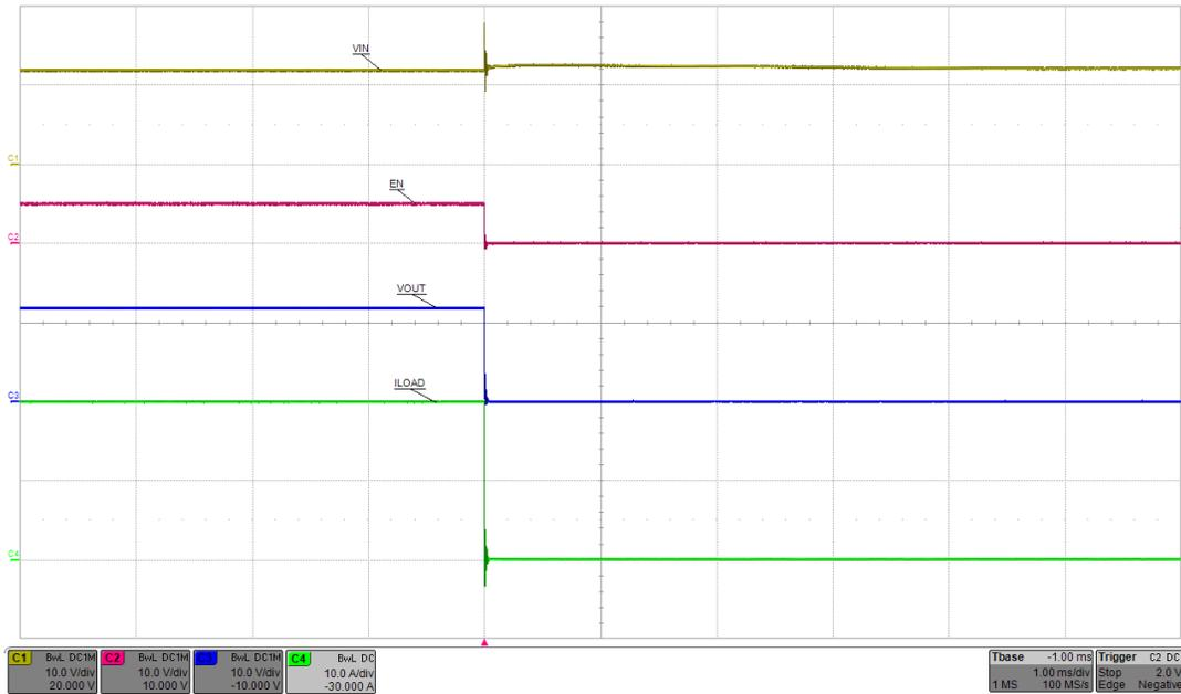
Figure 10. Load Turn-Off Behavior of 20-A eFuse With Enable-Off
