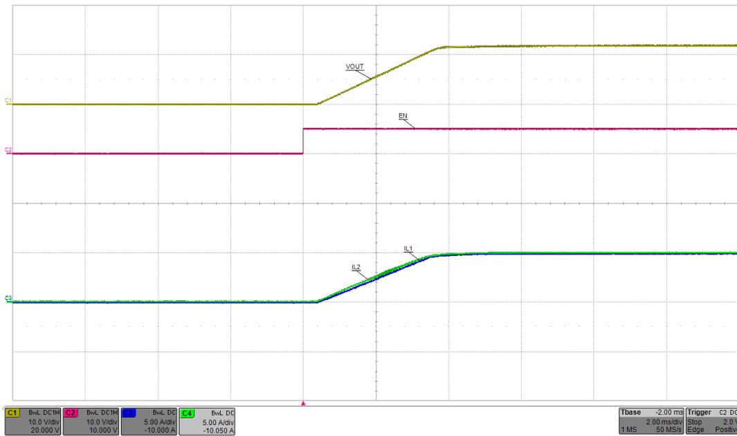
Figure 7. Current Sharing Among Two Devices During Output Voltage Ramp
