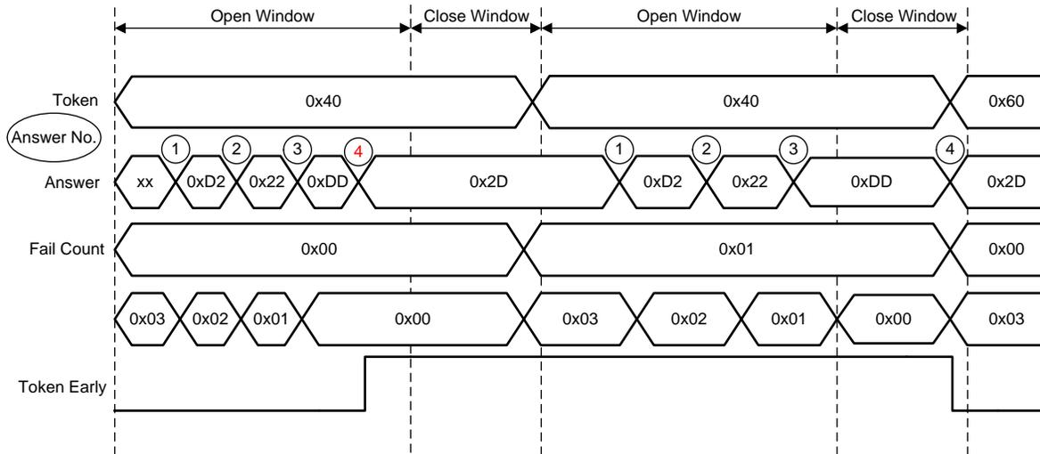
Figure 6. Out-of-Timing Window Timing Diagram
