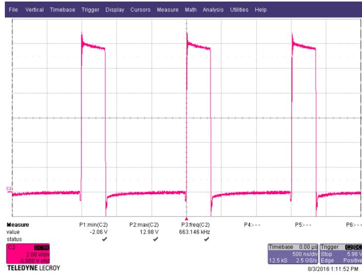
Figure 13. Switch Node Waveform – Layout 1
