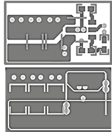
Figure 4. Layout 3 - Inductor + Output Capacitors on Other Side
