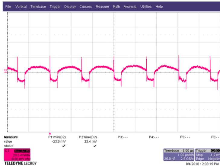
Figure 6. Output Ripple – 12 V to 2.5 V at 2.5 A. Layout 1
