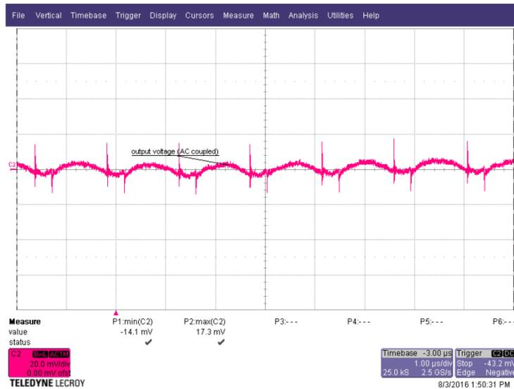
Figure 7. Output Ripple – 12 V to 2.5 V at 2.5 A, Layout 2
