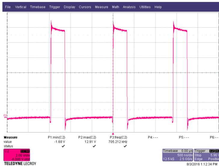
Figure 14. Switch Node Waveform – Layout 2
