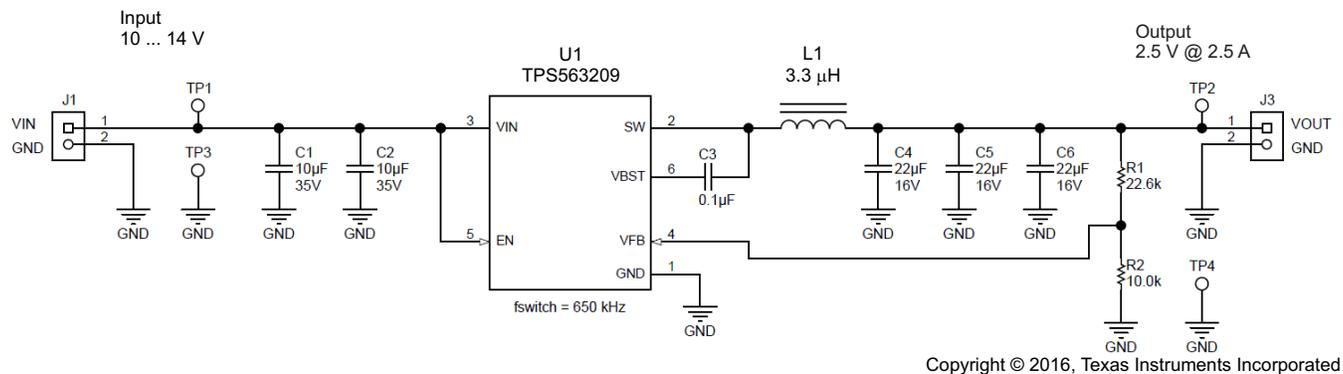
Figure 1. TPS563209DDCR 12 V to 2.5 V at 2.5 A
