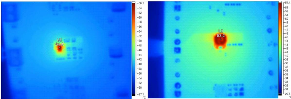
Figure 17. Layout 2 - IC Bottom Side (Left) Inductor Topside (Right)
