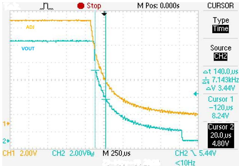
Figure 16. Switching Characteristics of the TPS7B4250-Q1 Device During Shutdown With a 50-mA Load,  $R_a = 10 \text{ k}\Omega$ ,  $C_a = 1 \text{ nF}$ ,  $R_o = 240 \Omega$ ,  $C_o = 10 \text{ nF}$
