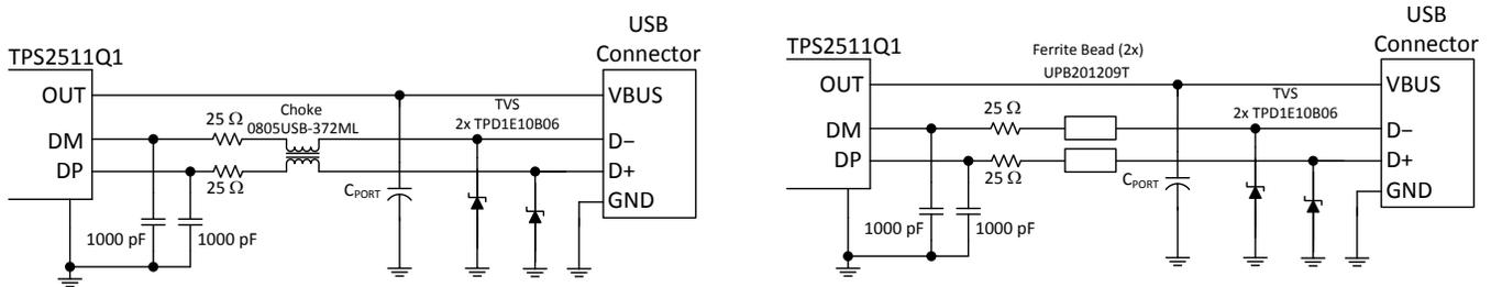
**Figure 4. Extended ESD Protection Circuit Examples**
