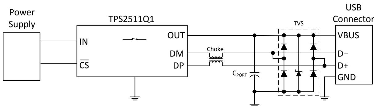
**Figure 1. Basic USB ESD Protection Circuit**
