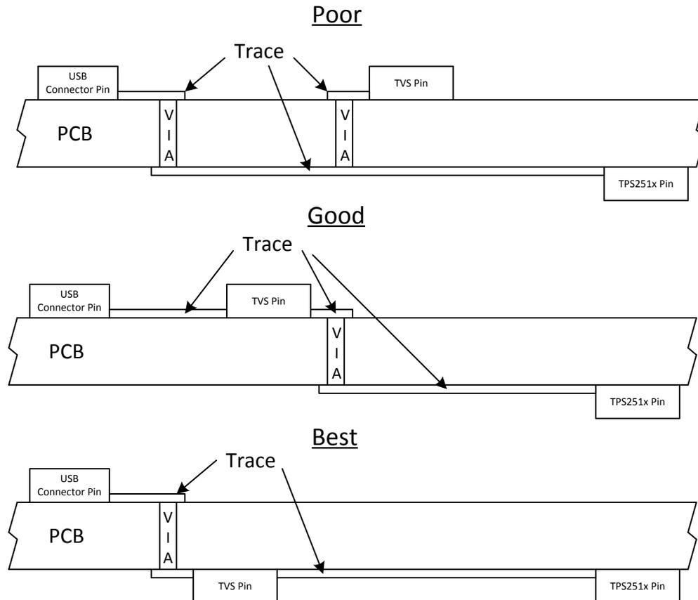
**Figure 3. Examples of TVS Placement and Connectivity**
