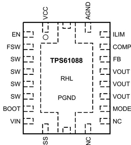
Figure 2. TPS61088 Pin Configuration
