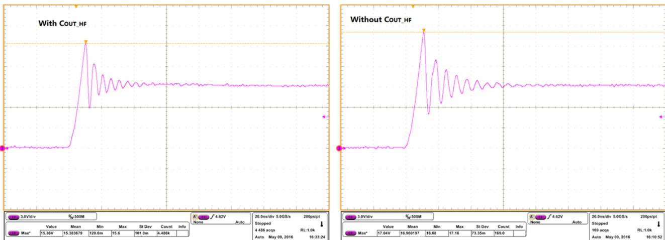
Figure 5. SW Voltage Spike With and Without  $C_{OUT\_HF}$
