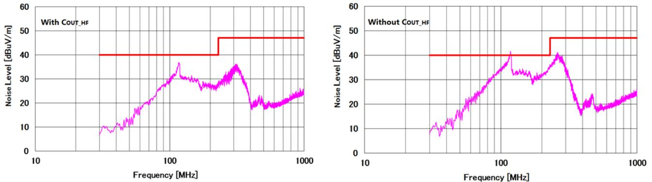
Figure 6. Radiated EMI Result With and Without  $C_{OUT\_HF}$
