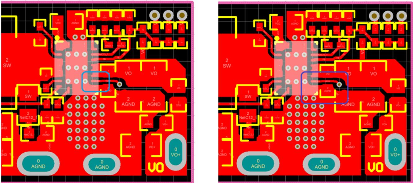
Figure 4. Critical Path Area With and Without  $C_{OUT\_HF}$
