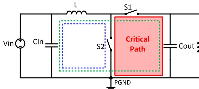
Figure 1. Critical Current Path of Boost Converter
