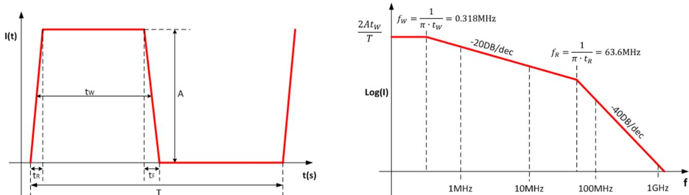
Figure 10. Harmonic Content of a Pulsed Current Waveform
