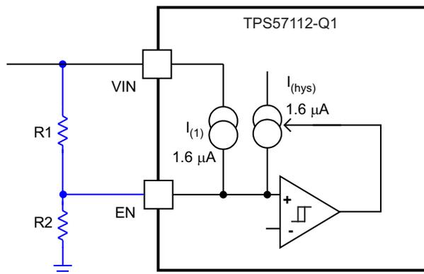
**Figure 1. Adjustable Undervoltage Lockout Using External Voltage Divider to VIN Pin**
