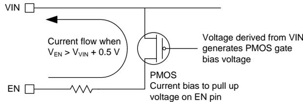
Figure 2. Internal Drive Structure of EN and VIN Pins
