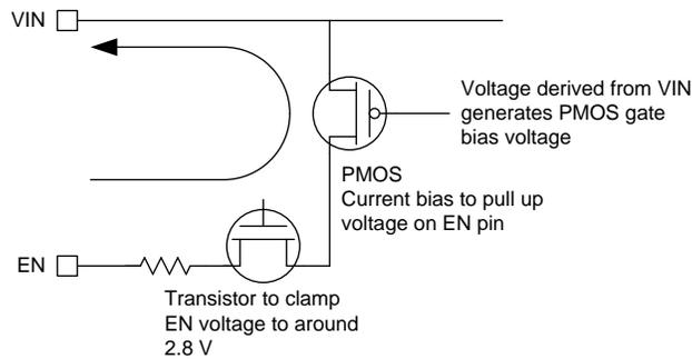
**Figure 4. Internal Drive Structure of EN and VIN Pins With PCN20140408000A**
