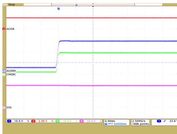
Figure 9. bq24770 Circuit Implementing PPS With ACDRV Control, ACDRV is Released and ACOK Remains High
