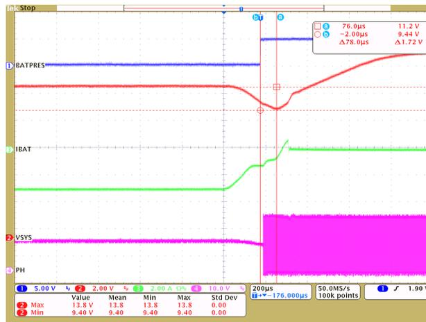
Figure 15. bq24770 Circuit Using LEARN Command, When LEARN Mode is Exit With Removing Battery and Releasing BATPRES HIGH
