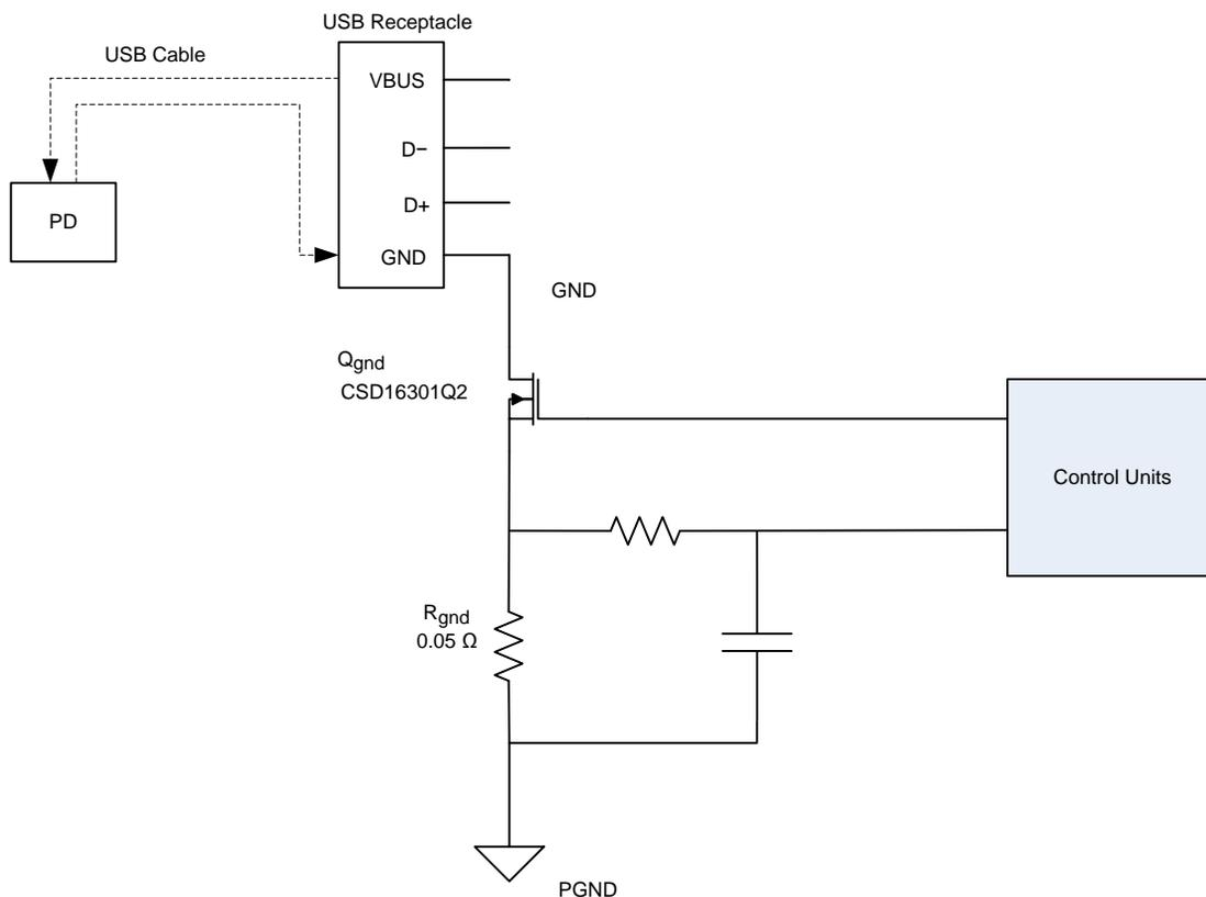
**Figure 4. Ground Return Path of a Power Bank**
