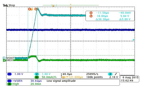
Figure 16. RCP TPS22953 Power Mux Activation Time
