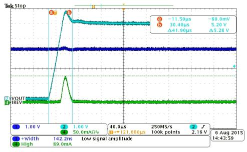
Figure 13. RCP TPS22963C Power Mux Leveling Time
