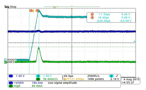
Figure 14. RCP TPS22963C Power Mux Activation Time
