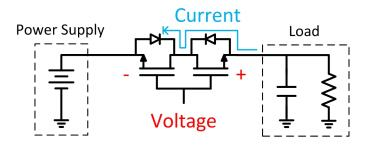
Figure 4. Reverse Current Blocking with Dual FETs
