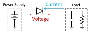
Figure 3. Reverse Current Blocking With a Diode
