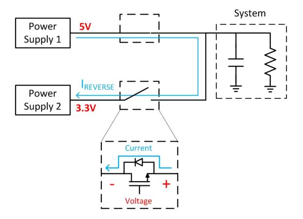
Figure 10. Reverse Current Caused by Power Muxing
