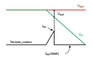
Figure 18. TPS2291xx Reverse Current Blocking Diagram
