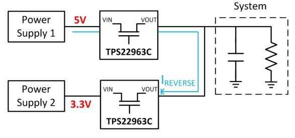
Figure 11. TPS22963C Reverse Current Blocking (5 V Closed, 3.3 V Open)
