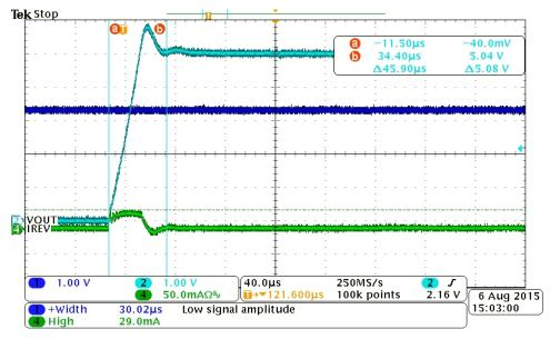
Figure 17. RCP TPS22953 Power Mux Leveling Time
