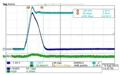
Figure 8. RCP TPS22963C V<sub>IN</sub> Leveling Time
