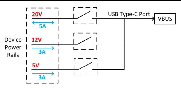
Figure 6. USB Type-C Power Muxing
