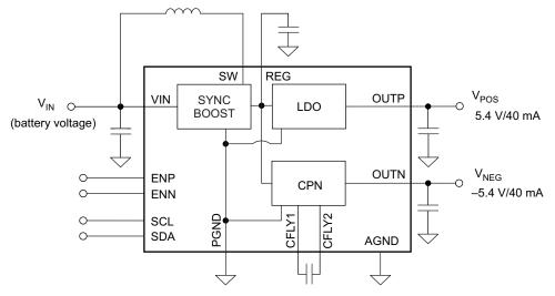
Figure 5. TPS65132 Block Diagram
