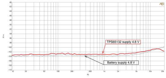
Figure 9. THD + N Battery Versus TPS65132
