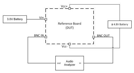
Figure 7. Test Setup
