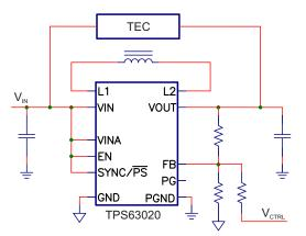
Figure 1. Circuit Schematic
