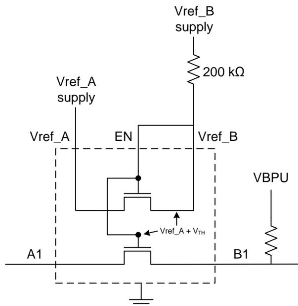
**Figure 1. Basics of LSF010x Theory of Operation**
