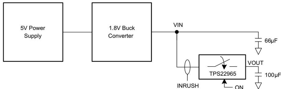
Figure 15. System Block Diagram utilizing the TPS22965
