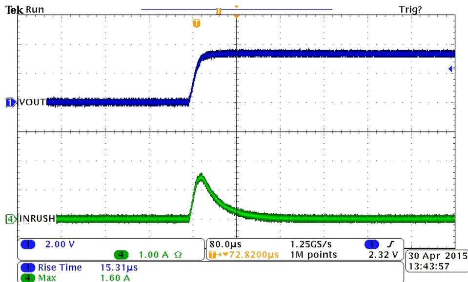
Figure 3. 3.3 V Applied to a 22  $\mu\text{F}$  Capacitor
