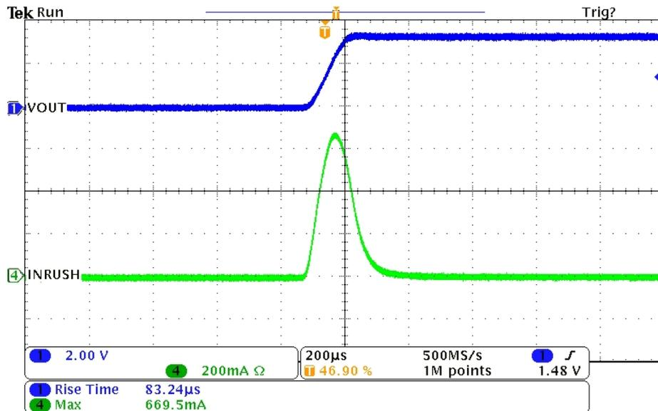
Figure 10. TPS22965 Scope Capture (CT cap = 0 pF)
