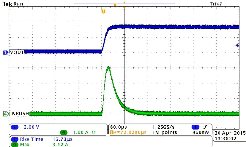
Figure 2. 3.3V Applied to a 47  $\mu\text{F}$  Capacitor
