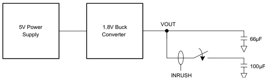
Figure 13. System Block Diagram without Slew Rate Control
