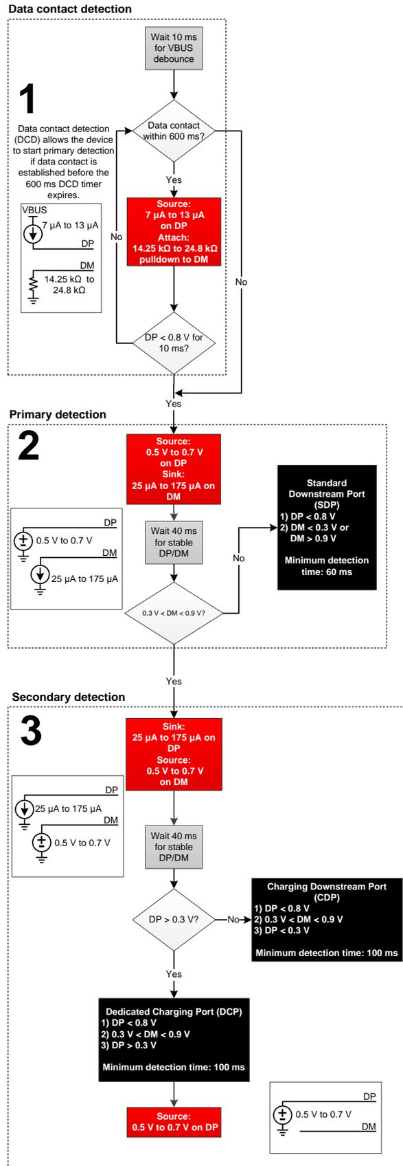
Figure 5. BC1.2 Charger Detection Flowchart
