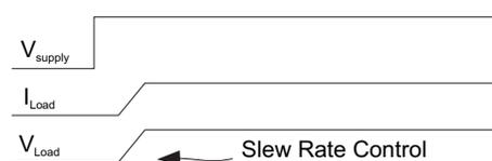
Figure 7. Slew Rate Control with Load Switch
