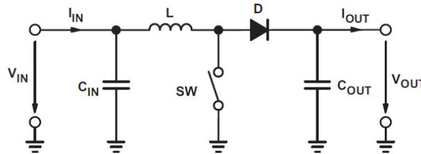
**Figure 1. Boost Converter Circuit**
