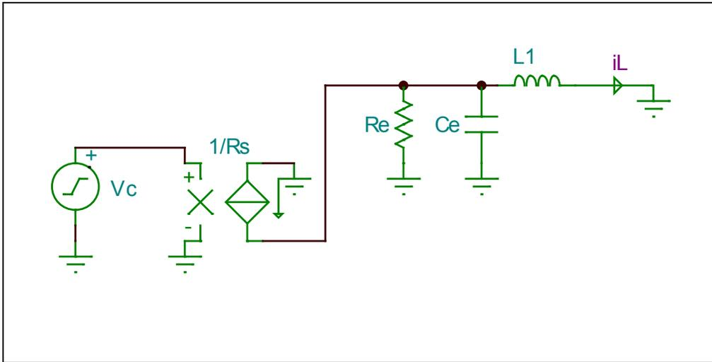
**Figure 2. Gain from Control to Inductor Current**
