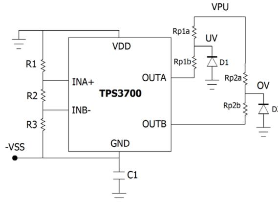
Figure 1. Monitoring a Negative Voltage Rail Using the TPS3700
