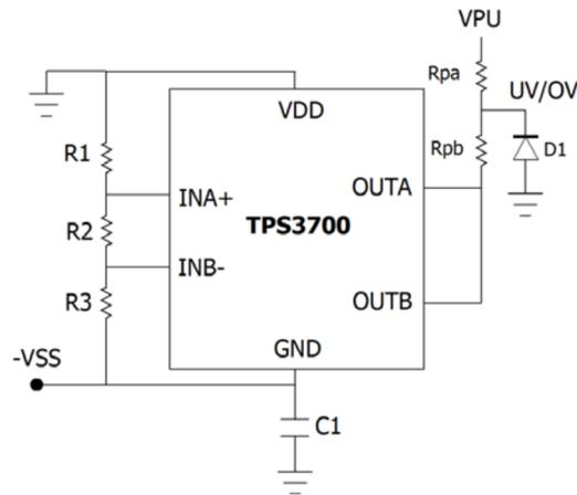
Figure 3. Wired-OR Output Configuration
