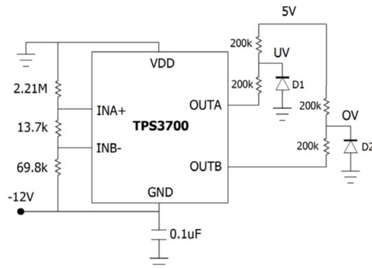
Figure 4. TPS3700 Negative Monitoring Design Example
