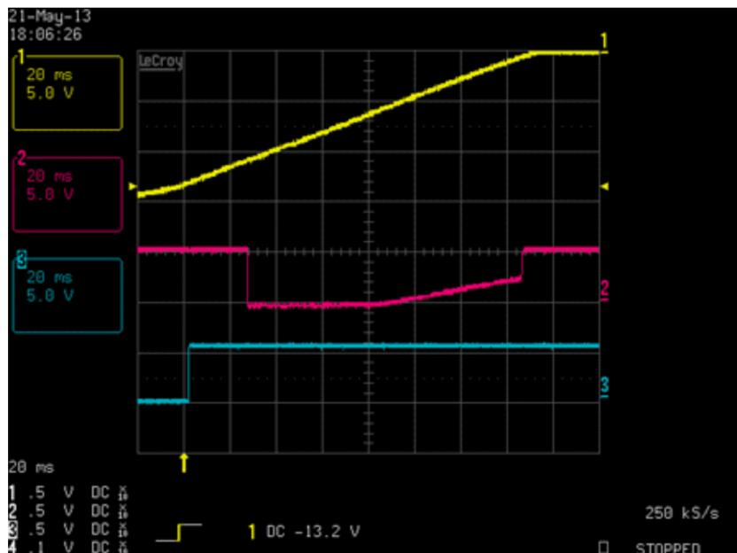
Figure 6. OUTA and OUTB Response for VDD Voltage Falling
