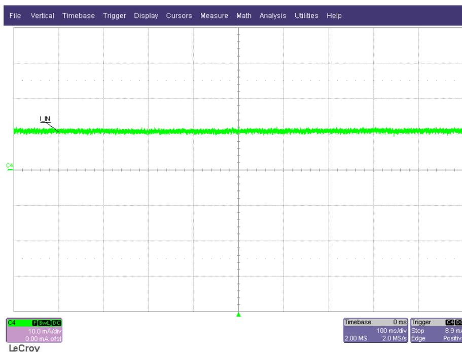
**Figure 10. Input Current in Sleep Mode with MODE High**
