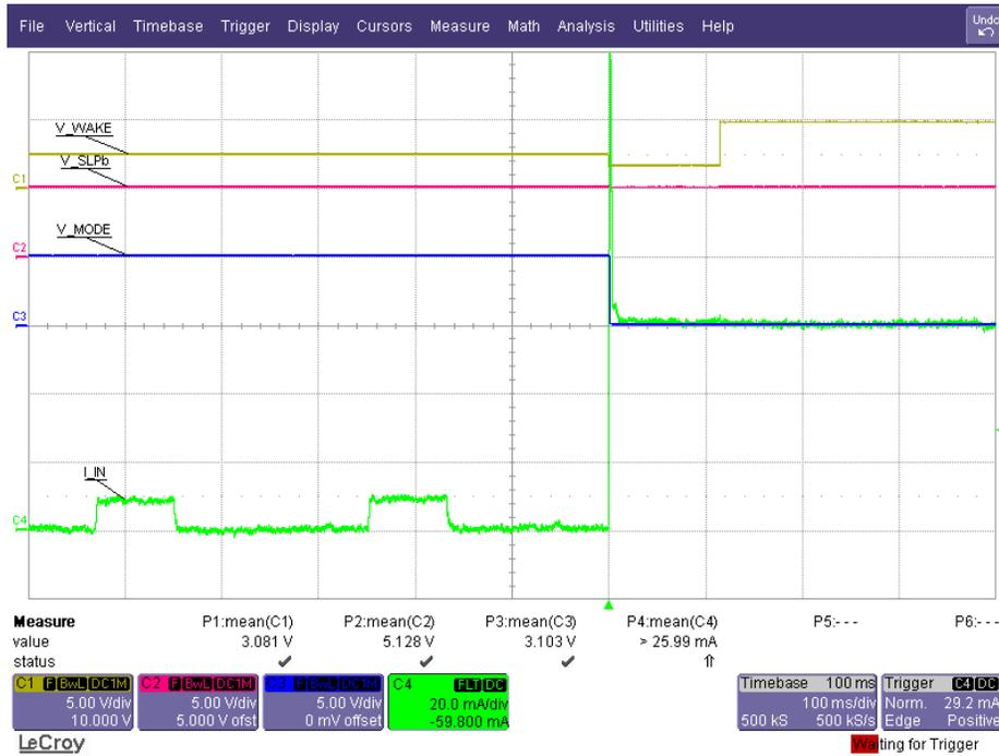
Figure 11. Exiting Sleep Mode with MODE Low and SLPb High
