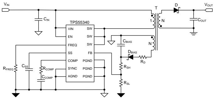
Figure 10. Isolated Flyback with Bias Winding
