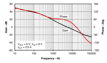
Figure 7. Total Loop Small Signal Response
