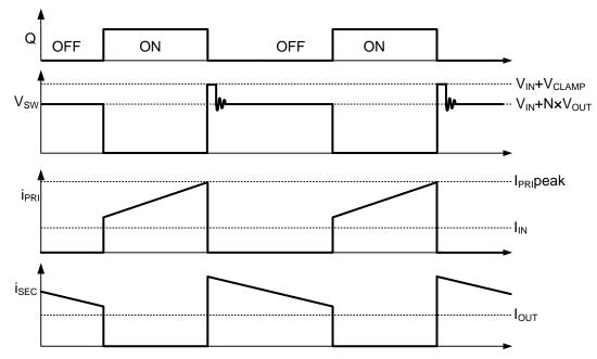
Figure 2. CCM Flyback Voltage and Current Waveforms
