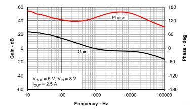
Figure 6. Compensation Small Signal Response
