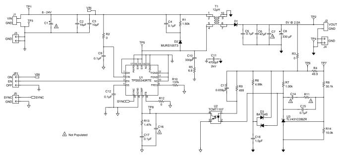
Figure 1. Reference Design Schematic
