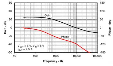
Figure 5. Power Stage Small Signal Response
