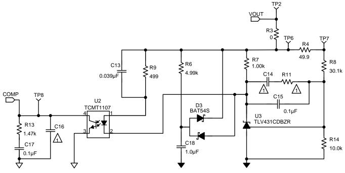
Figure 3. Opto-Coupler and Feedback Circuitry
