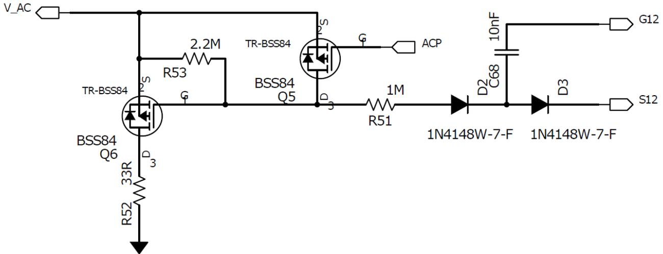
Figure 6. AC Adapter (V\_AC) Capacitor Discharge Circuit
