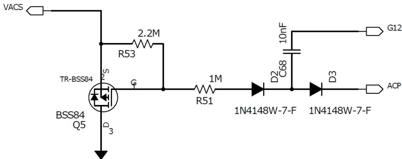
Figure 3. AC Adapter Sense (VACS) Discharge Circuit
