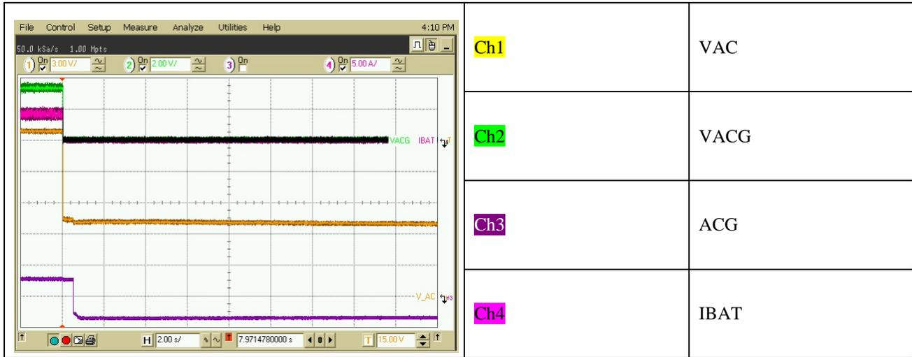
Figure 5. Oscilloscope Plot of VACS Discharge
