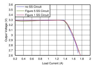
Figure 10. Load Regulation Effect of the Soft Start Circuits
