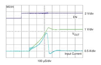
Figure 2. TPS63010EVM With Extra Output Capacitance Soft Starting Into 100- $\Omega$  Load – 250- $\mu$ S Soft Start Time and 1.4 A of Inrush Current
