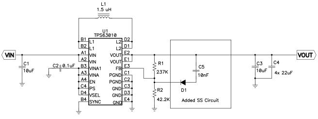
Figure 1. TPS63010EVM With Added Soft Start Circuit
