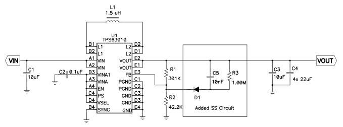
Figure 5. TPS63010EVM With Alternative Soft Start Circuit
