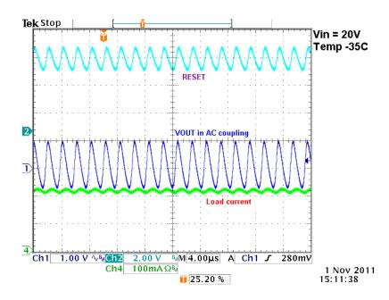
Clearly the voltage does not meet the requirements for stable, well regulated 5V output.
