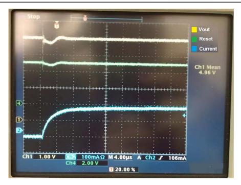
Figure 2.  $68\mu\text{F}/16\text{V}$  Panasonic EEE-FT Series Cap at  $V_{\text{IN}}$  = 20V
