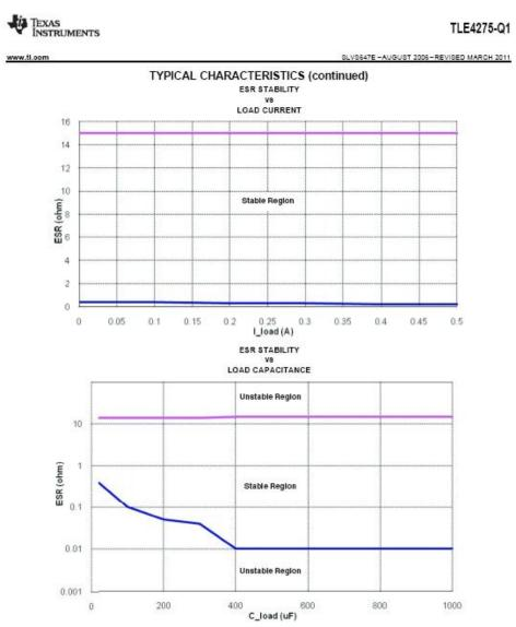
System designs must ensure their capacitor choice meets the published ESR limits for TLE4275 stability. When ceramic capacitors are used, a series resistor may be required to meet resistance minimum value. As an example, a 22  $\mu F$  ceramic capacitor with a .33- $\Omega$  series resistor will meet stability requirements over full temperature range.
