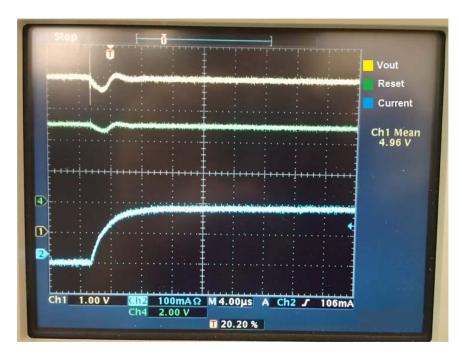
Figure 1.  $68\mu F/16V$  Nichicon UD Series Cap at  $V_{IN} = 20V$
