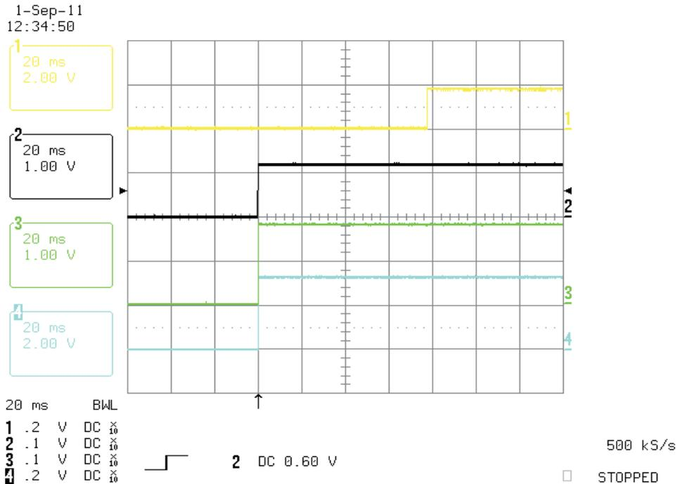
Figure 4. TPS650061 Power-On and /Reset Ch1-/RST, Ch2-VODC, Ch3-VLDO2, Ch4-VLDO1
