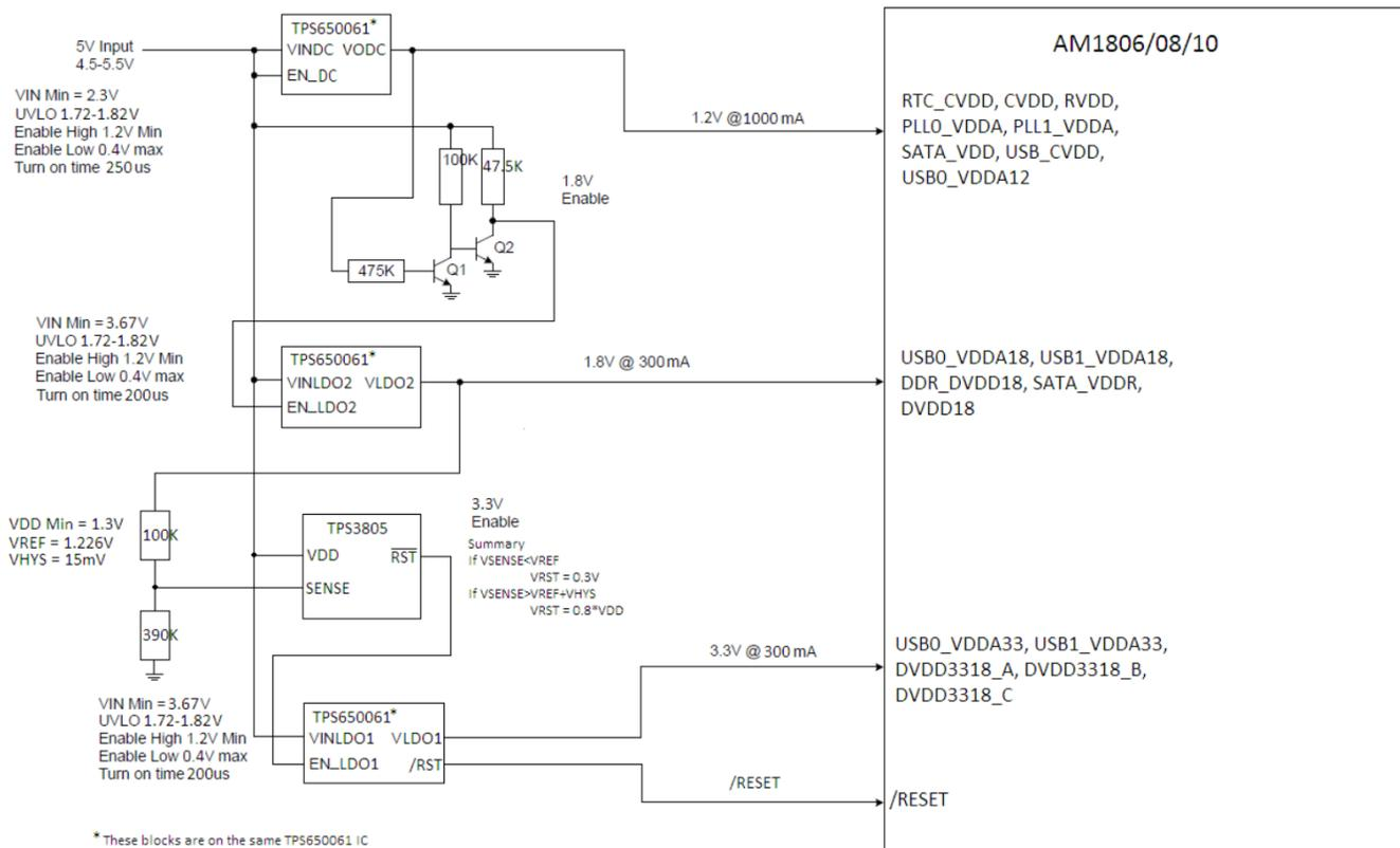
Figure 1. TPS3805, TPS650061, and AM1806/08/10 Block Diagram
