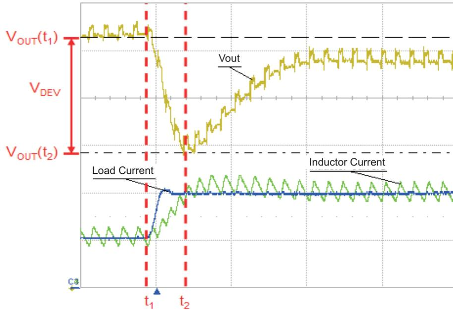
Figure 1. Load Transient Response of the TPS62130
