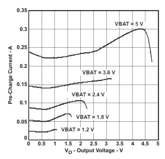
Figure 3. Short-Circuit Precharge Current
