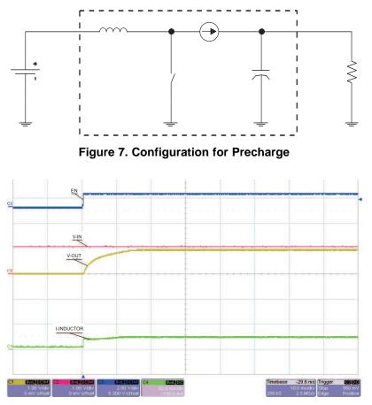
Figure 8. TPS61020 Start-Up Stuck in Precharge, Load 45  $\Omega$
