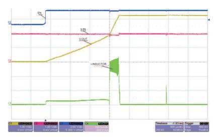
Figure 5. TPS61020 Start-Up From 2 V
