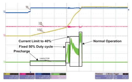
Figure 4. TPS61020 Start-Up From 1 V
