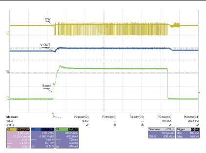
Figure 7. Load Transient (0 mA to 500 mA)
