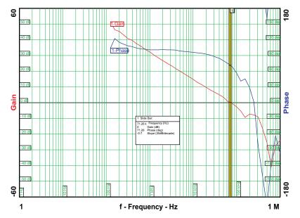
Figure 6. Loop Gain Measurements (PM = 71.26 deg, Fco = 71.26 kHz)
