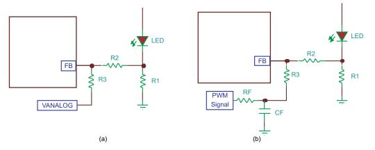
Figure 3. Analog Dimming Using (a) Variable DC voltage (b) PWM Signal
