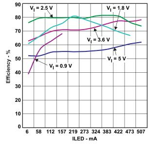
Figure 4. Efficiency vs VIN Graphs
