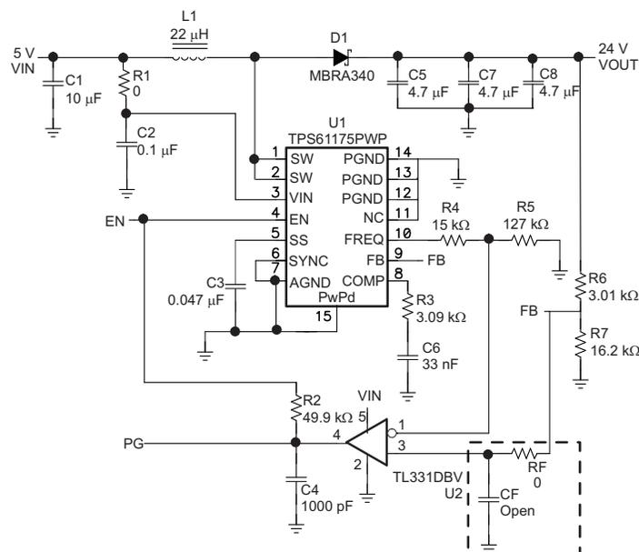
Figure 1. TPS61175 With PG Circuit Using the TL331
