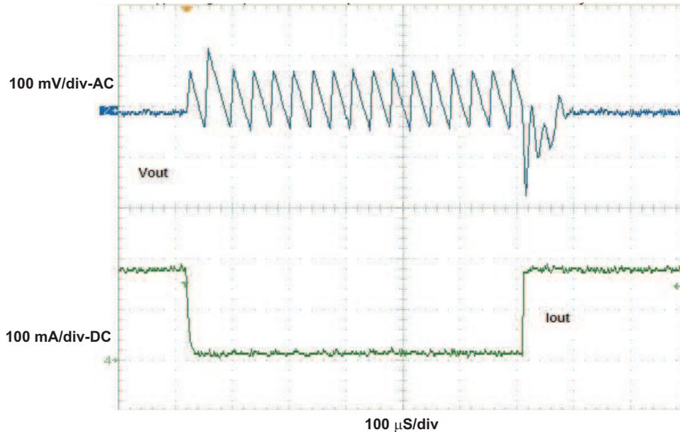
Figure 5. TPS61070EVM Transient Response Without Soft Start Circuit
