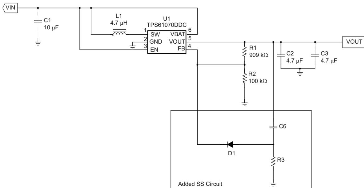
**Figure 1. TPS61070EVM With Added Soft Start Circuit**
