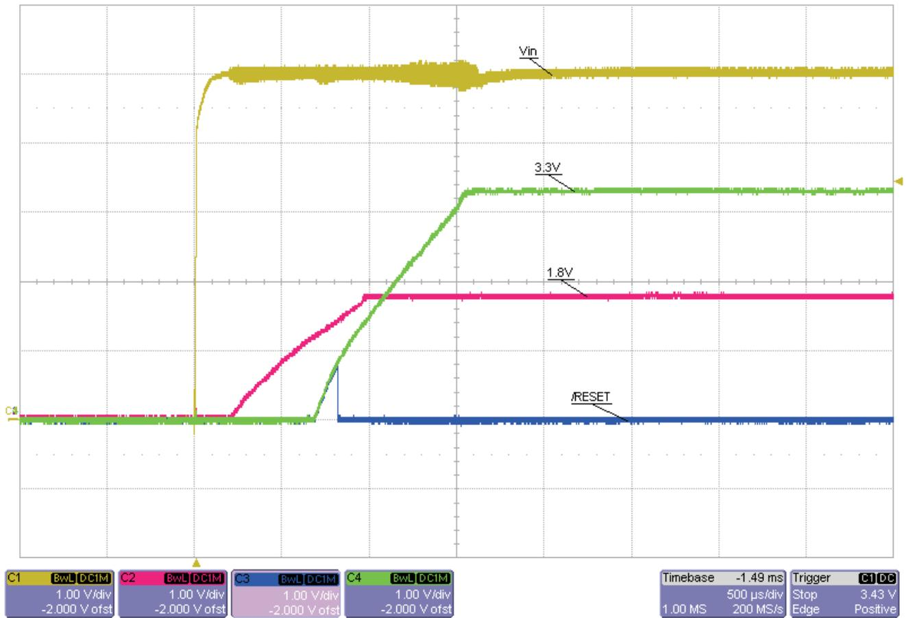
Figure 2. The 1.8-V Rail Voltage Rises Before the 3.3-V Rail
