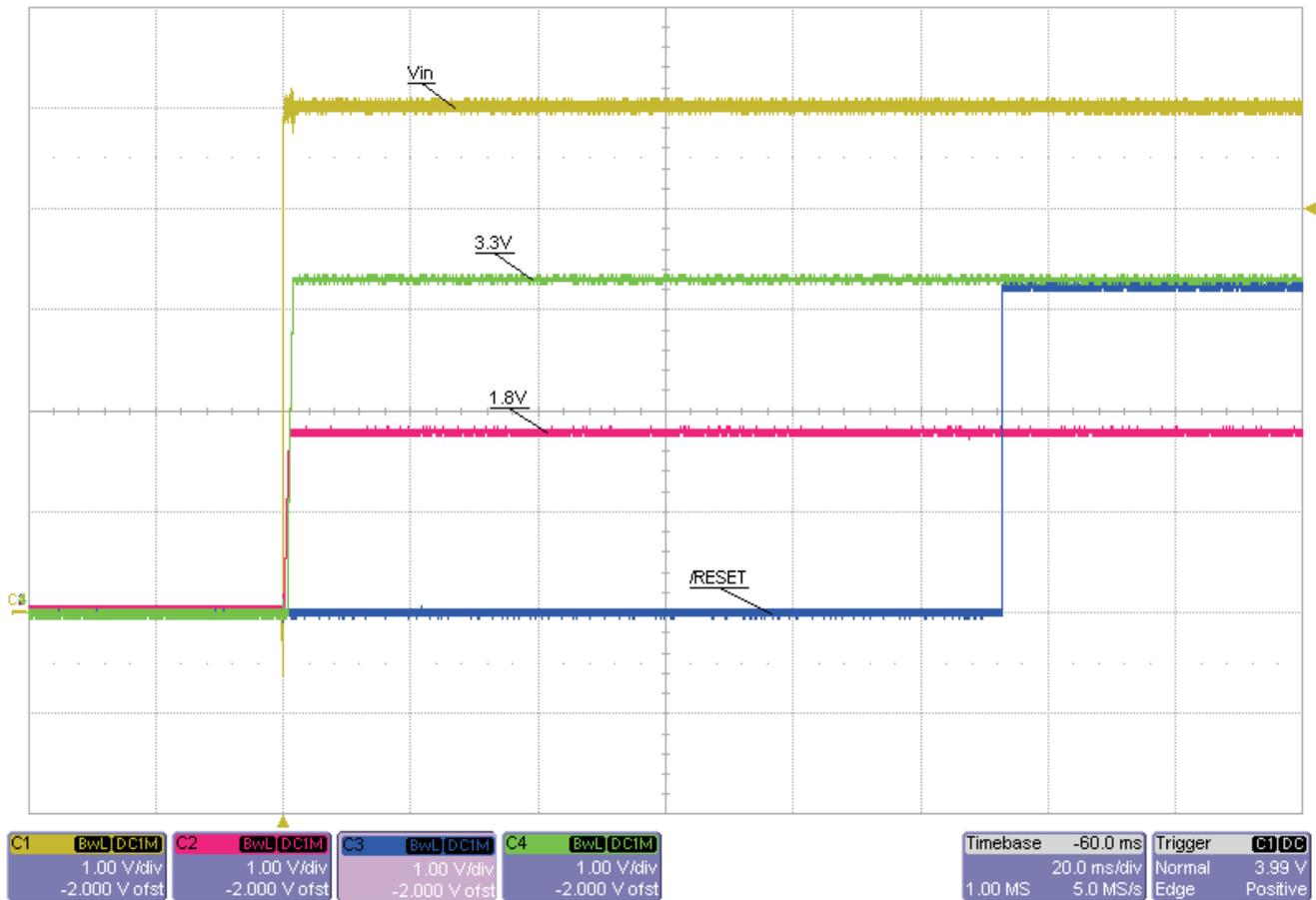
Figure 3. The RESET Signal Held Low for a 100-ms Typical Fixed Delay
