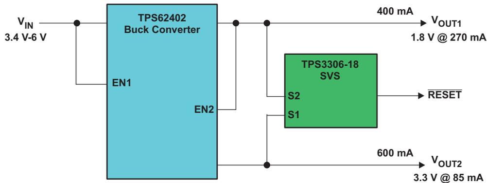
**Figure 1. Block Diagram of Power Design**
