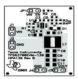
Figure 4. Inverter Improved Board Layout
