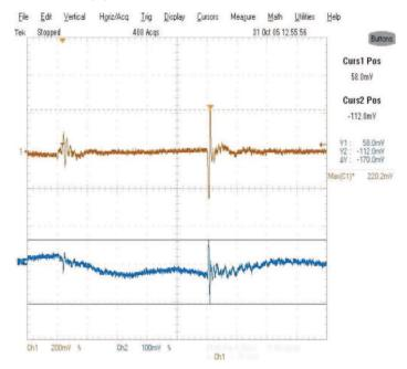
Figure 5. High-Frequency Switching Noise on Output of Inverter Using Improved Board Layout and Bypass Capacitors
