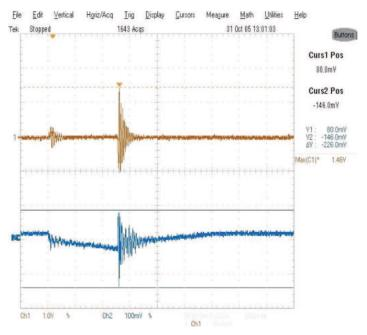
Figure 1. High-Frequency Switching Noise Measurement Using Bad Board Layout
