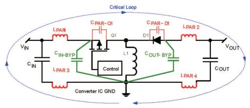
Figure 3. Buck-Boost (Inverting) Converter Schematic
