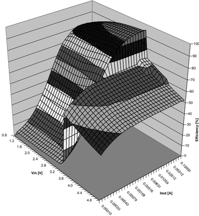
Fig. 9. Efficiency for  $V_{out} = 3.3V$  with power save mode disabled.
