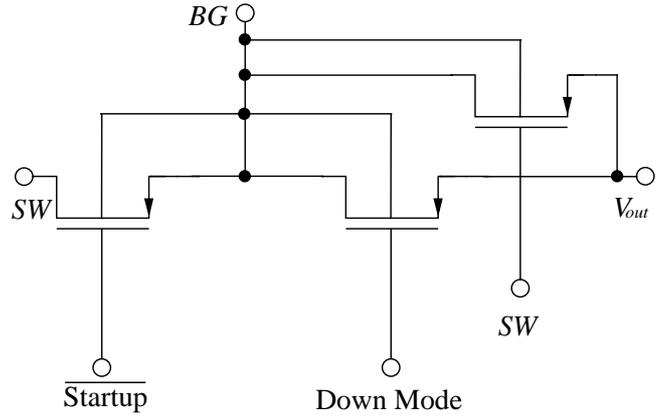
Fig. 6. Back-gate control switches .
