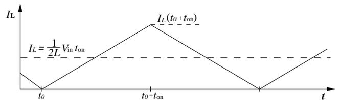
Fig. 4. Inductor current at border from continuous mode to power save mode.
