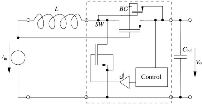
Fig. 5. Schematic of the converter in *down mode*.
