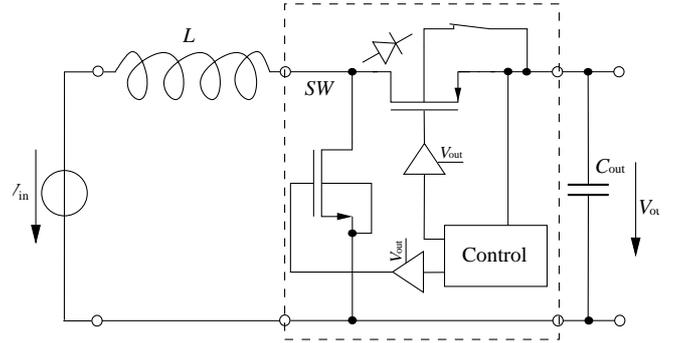
Fig. 3. Schematic of the converter in boost mode.
