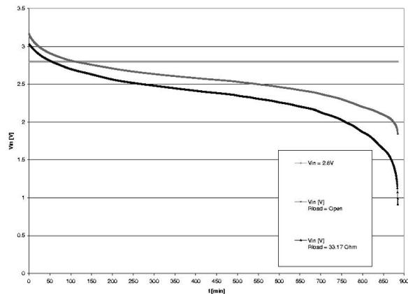
Fig. 1. Discharging of two alkaline cells in series at a boost converter input.
