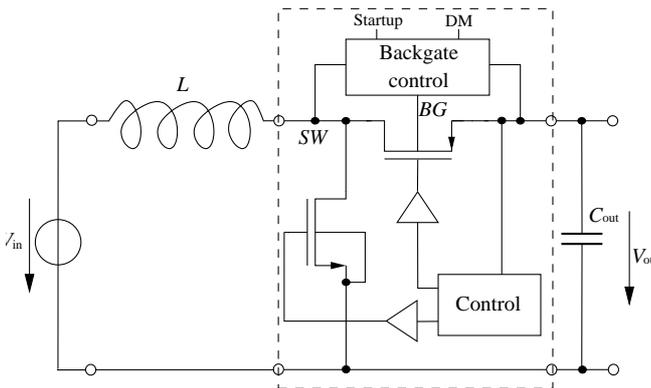
Fig. 2. Block diagram of the boost converter with down conversion capability.
