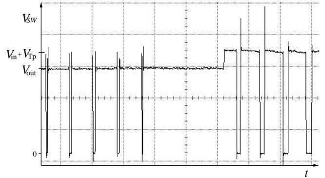
Fig. 7. Signal at  $SW$  at the changeover from boost mode (left) to down mode.
