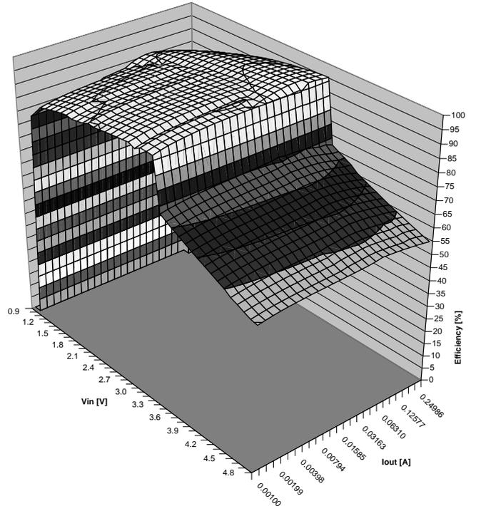
Fig. 10. Efficiency for  $V_{out} = 5.5V$  with power save mode enabled.
