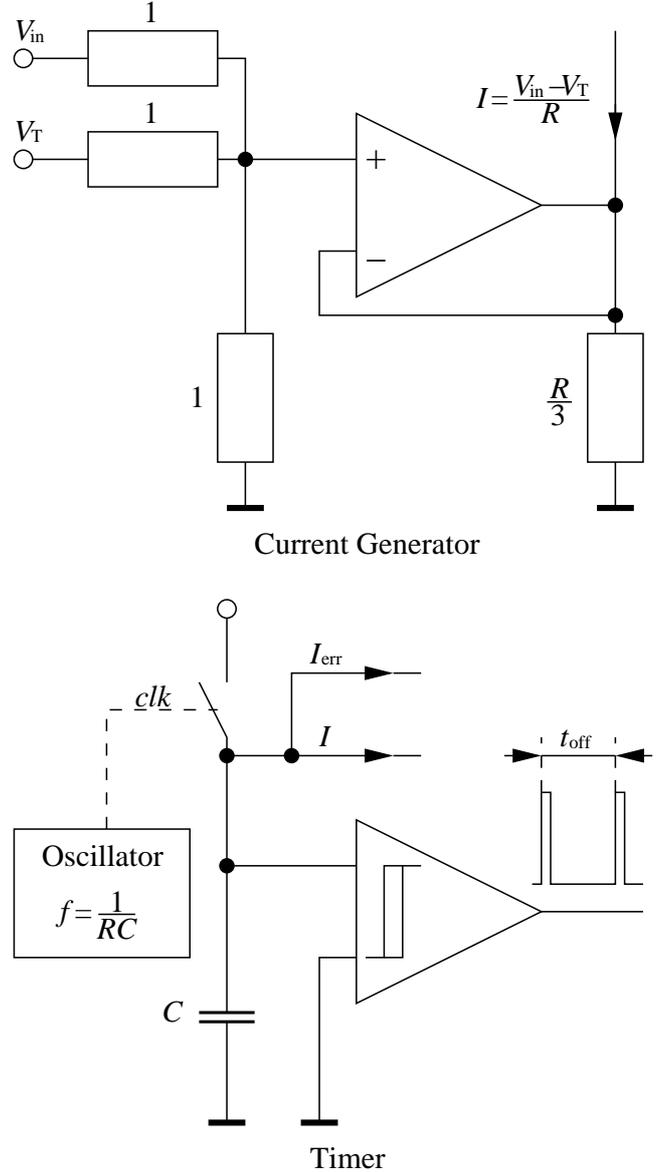
Fig. 8. Controller scheme for down mode.
