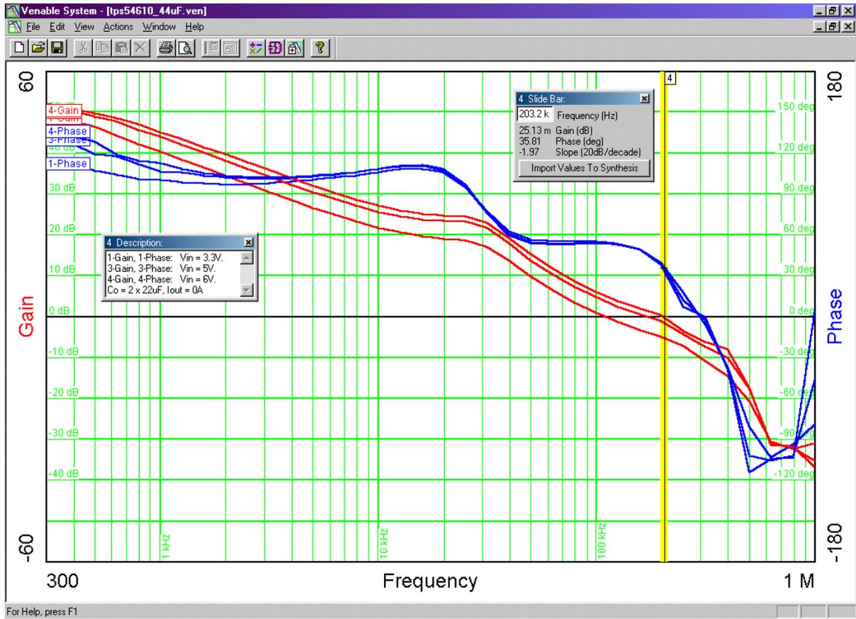
**Figure 6. Gain and Phase at No-Load With  $C_O = 44 \mu\text{F}$  (33% Less)**
