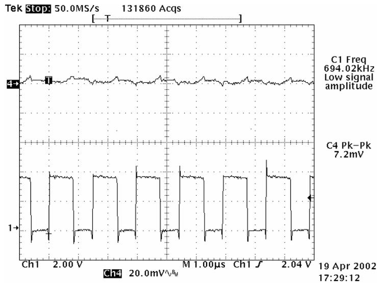
**Figure 2. Output Ripple and Switching Waveforms With 3 x 22- $\mu$ F Ceramic Capacitors**
