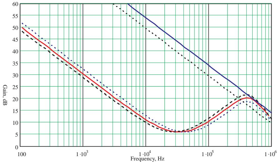
Dotted and solid lines to the right show minimal and typical envelope of error amplifier
