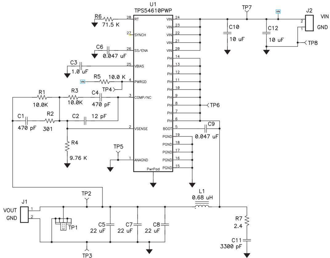
Figure 1. Electrical Schematic of Evaluation Module TPS54610EVM-213
