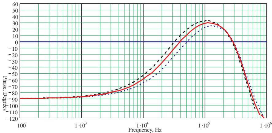
**Figure 14. Compensation Circuit Phase Including  $\pm 20\%$  Variations of Capacitors C1, C2, and C4**
