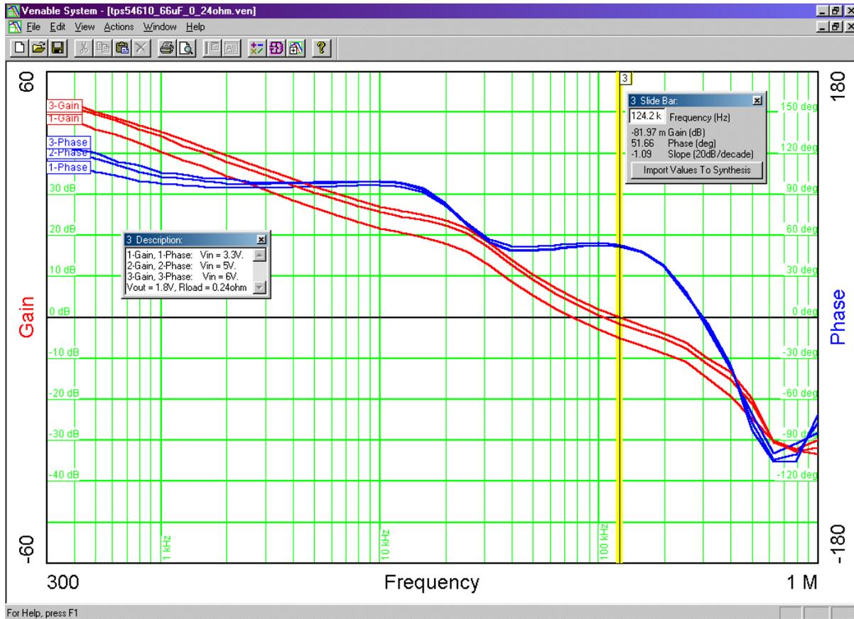
**Figure 5. Gain and Phase at  $R_L = 0.24 \Omega$  ( $I_O = 7.5 \text{ A}$ ) With  $C_O = 66 \mu\text{F}$**
