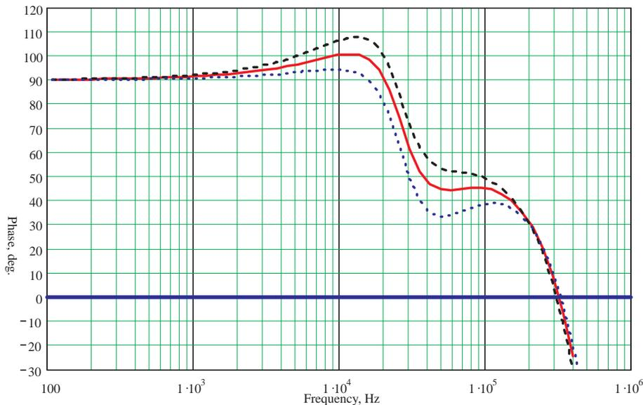
**Figure 12. Phase at 6-V Input Including  $\pm 20\%$  Variations of Capacitors C1, C2, and C4**
