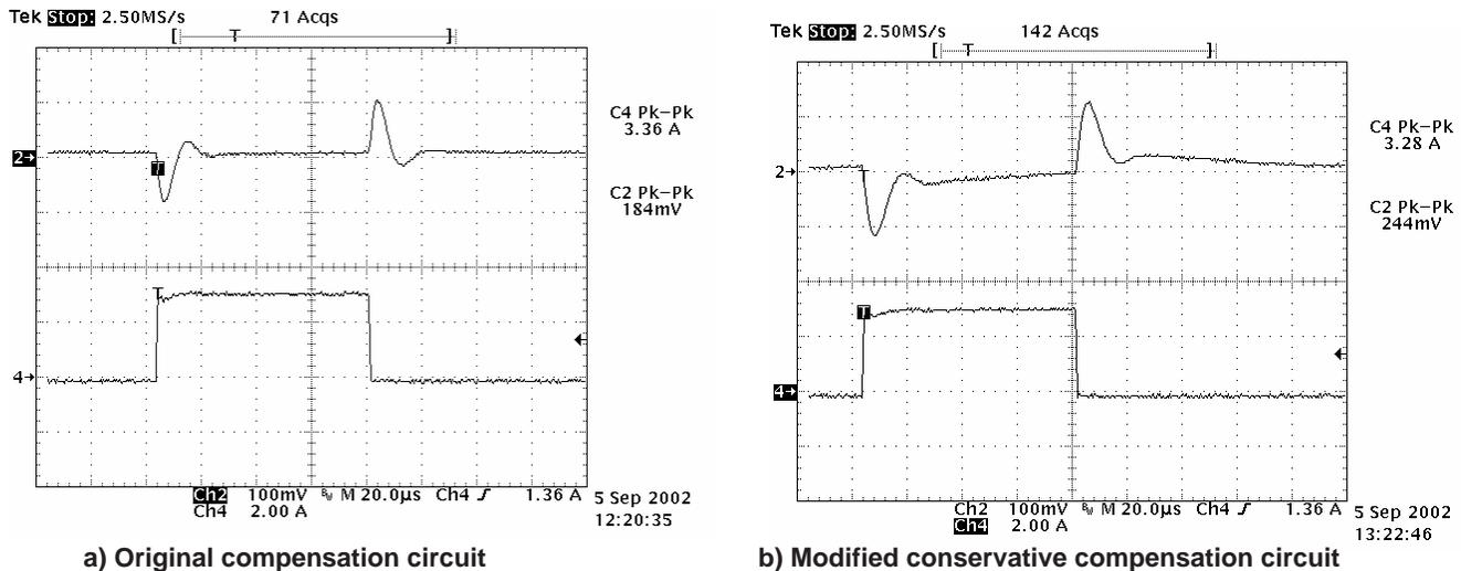
**Figure 20. Transient Response With the Original (a) and Modified (b) Compensation Circuit**
