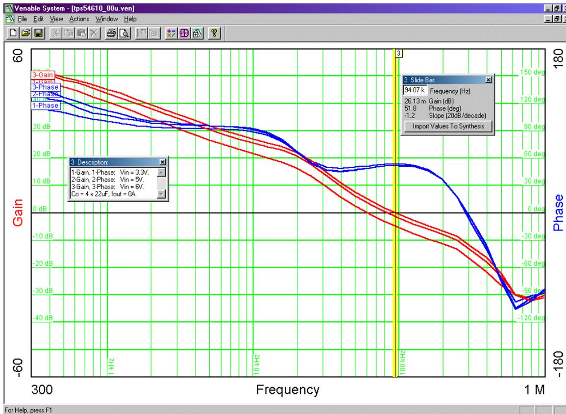
**Figure 7. Gain and Phase at No-Load With  $C_O = 88 \mu\text{F}$  (33% More)**
