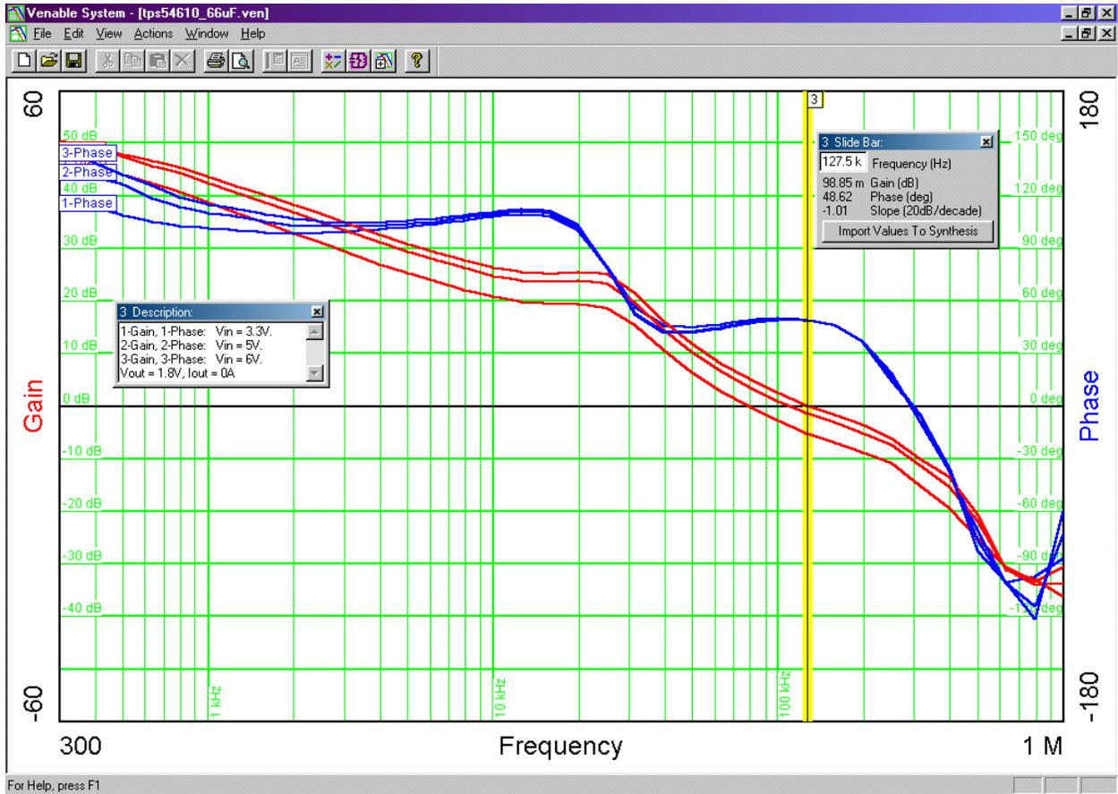
**Figure 4. Gain and Phase at No-Load Condition With  $C_O = 66 \mu\text{F}$**
