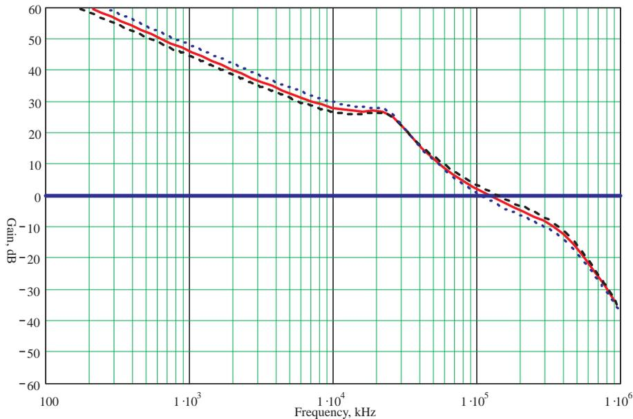
**Figure 11. Gain at 6-V Input Including  $\pm 20\%$  Variations of Capacitors C1, C2, and C4**
