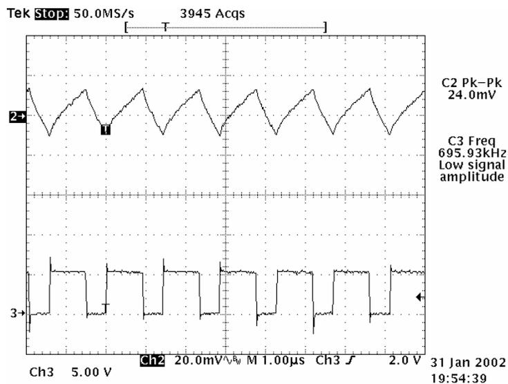
**Figure 3. Output Ripple and Switching Waveforms With 2 x 150- $\mu$ F SP-Type Capacitors**
