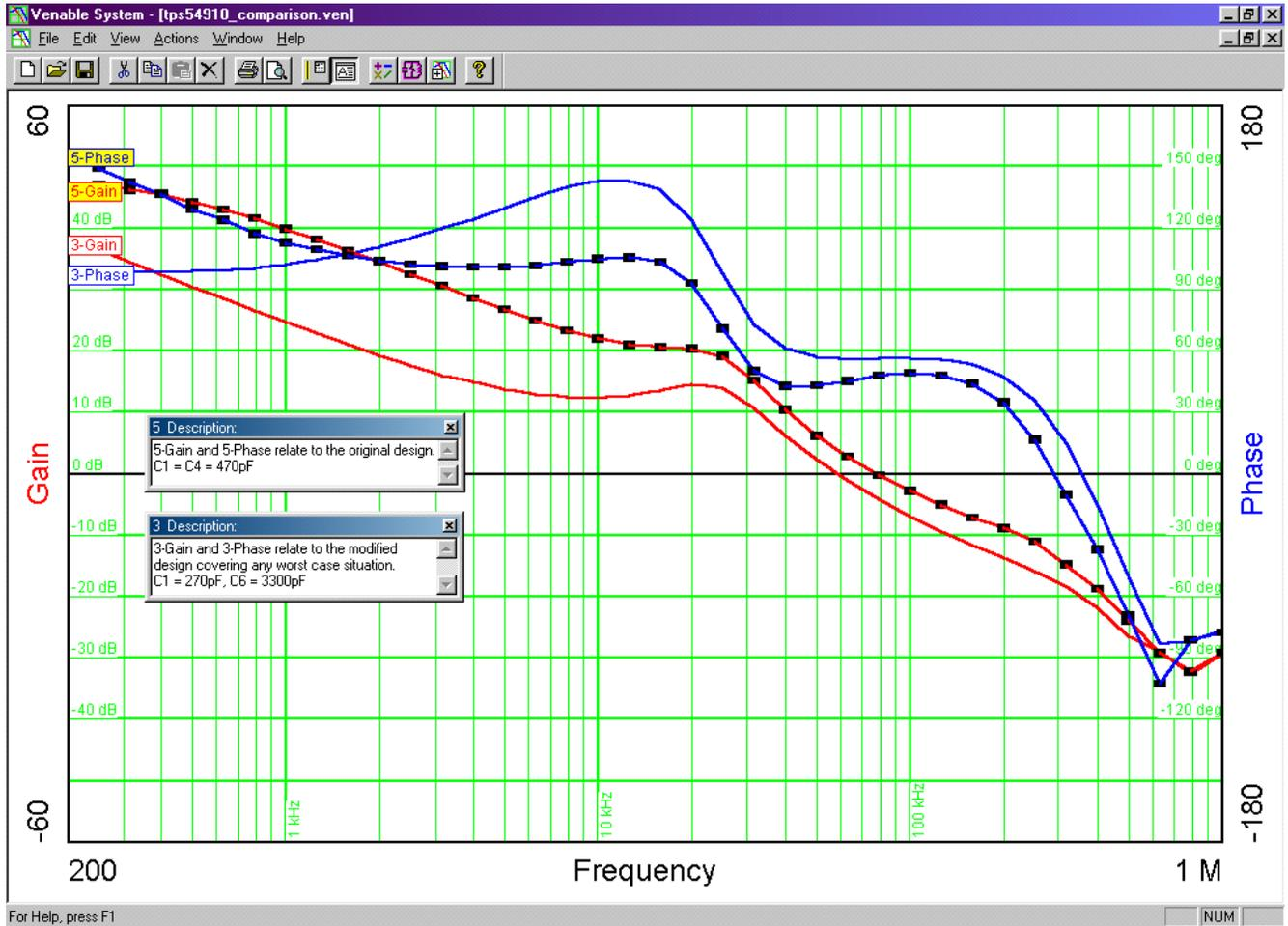
For the original compensation  $C1 = C4 = 470 \text{ pF}$ , for the modified compensation  $C1 = 270 \text{ pF}$ ,  $C4 = 3300 \text{ pF}$
