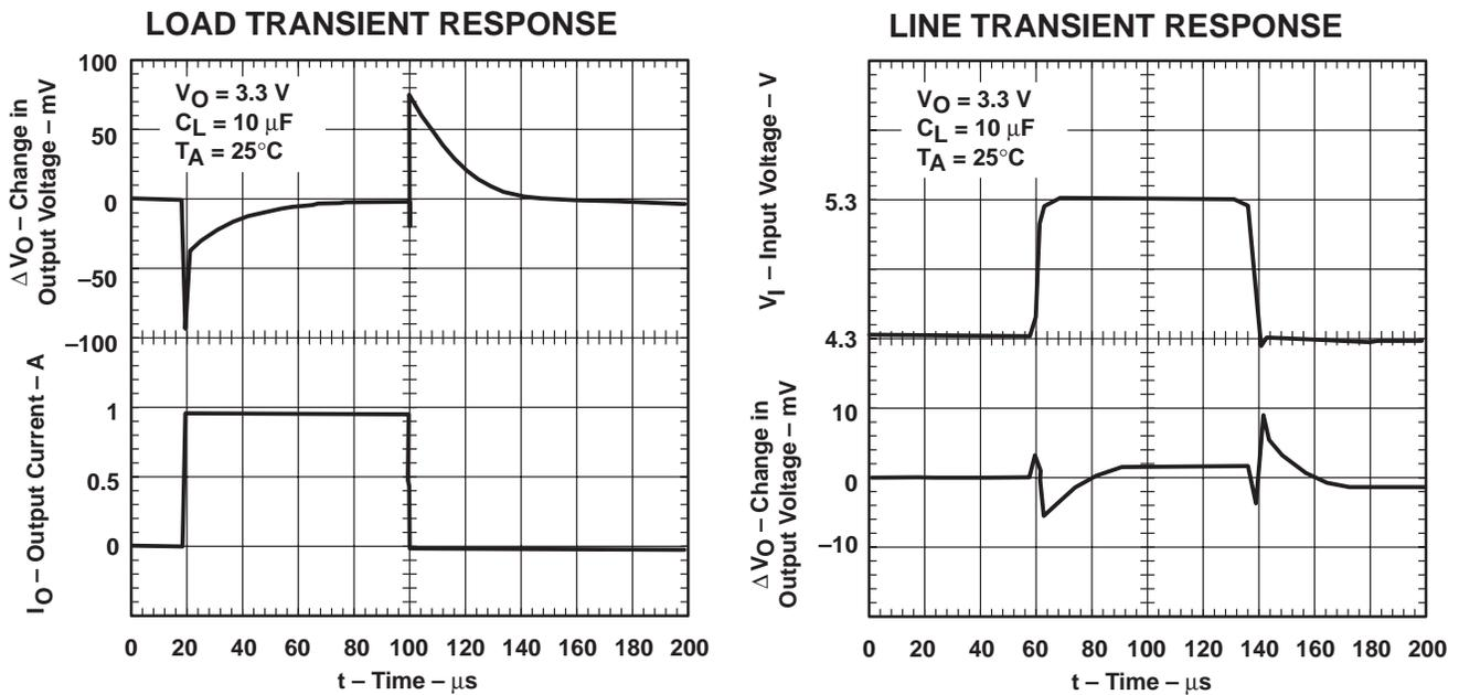
Figure 3. Graphics of Typical Current Transient Response of the 3.3-V Supply Output
