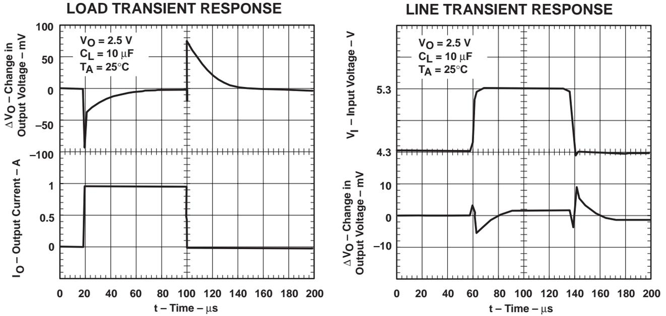
Figure 2. Graphics of Typical Current Transient Response of the 2.5-V Supply Output
