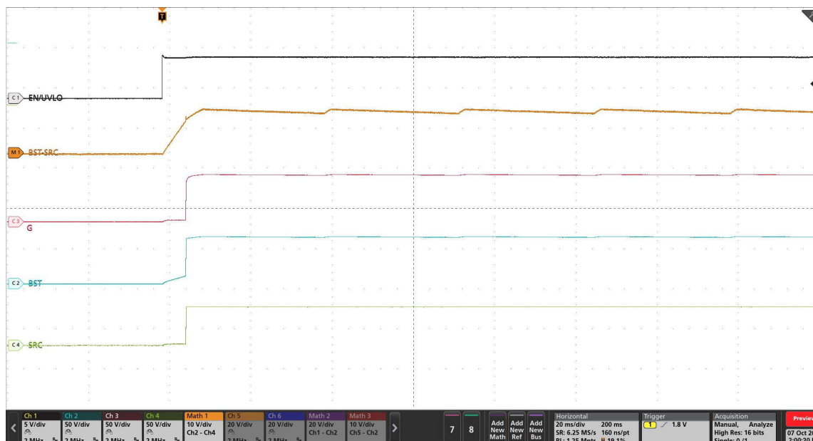
Figure 3-2. Start-Up Profile of Low Power Path ( \overline{\text{LPM}} = \text{LOW} , V_{\text{IN}} = 48\text{V} , No Load, C_{\text{BST}} = 470\text{ nF} )
