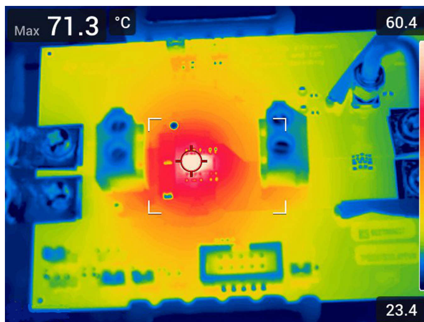
Figure 4-1. Thermal Performance (TPSM8287B30LAPEVM, V_{IN} = 5V , V_{OUT} = 0.6V , I_{OUT} = 30A )
